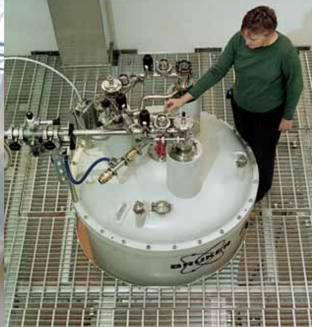
A protein sample being placed in the new £2 million 800MHz spectrometer, in order to determine its structure.
