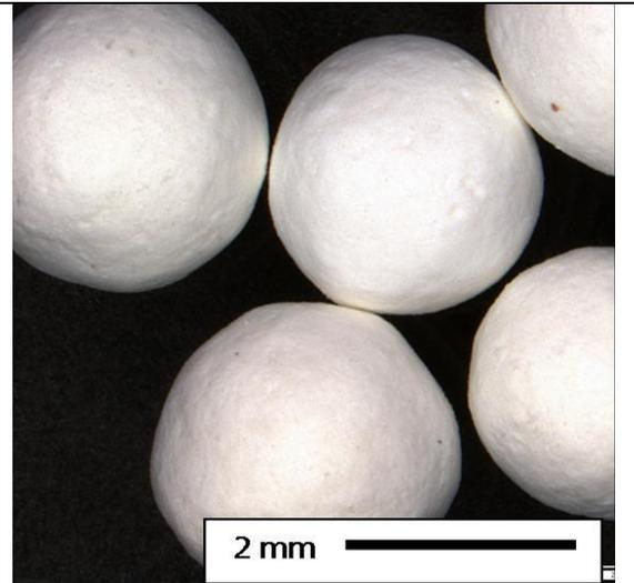
Fig. 2 Catalyst ( $\text{ZnO}$ ), prepared by fluidized bed granulation
