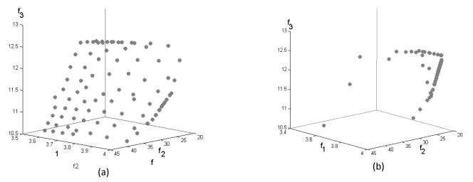
Fig. 10. Solutions obtained using (a) DBEA-Eps (b) MOEA/D-PBI on three-objective car side impact problem
