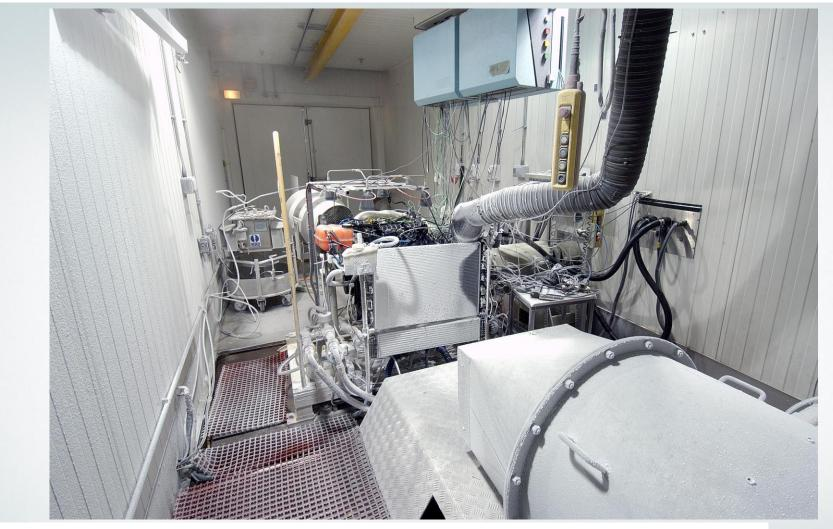
Dynamic dynamometer encapsulated test facility – can provide efficient, cost effective and realistic testing on a rig as opposed to building expensive prototype vehicles, which require specialised vehicle-based test facilities or testing in remote cold climate locations.
