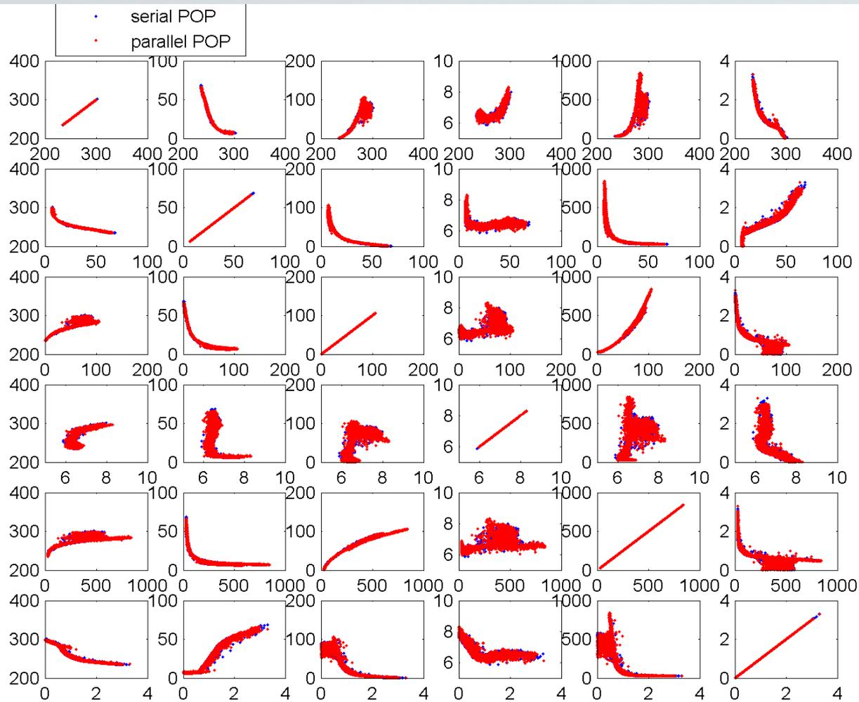
Pareto-optimal populations resulting from runs with serial and parallel versions of NSGAI. Objective axes not labelled for compactness and as they are not required.
