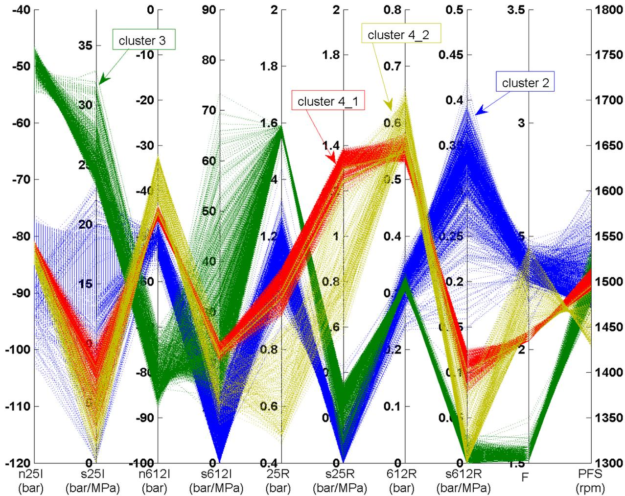
Parallel Coordinates plot of the final populations resulting from objective reduction in each cluster. The objectives have been re-ordered so that each sensitivity objective is adjacent to the objective to which it relates.
