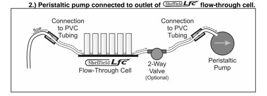
In this configuration, the sample is drawn entirely under suction through the <u>Sheffield</u> Lfc<sup>\*</sup> flow-through cell.
