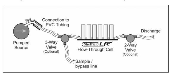
The Sheffield Lfc cell has been designed for use with low-flow pumping rates optimised between 0.5 and 1.0 litre/minute and a maximum flow rate of 1.5 litres/minute.
