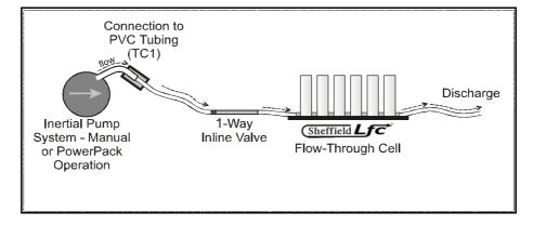
1.) Inertial pump system connected to Sheffield Lfc flow-through cell.
