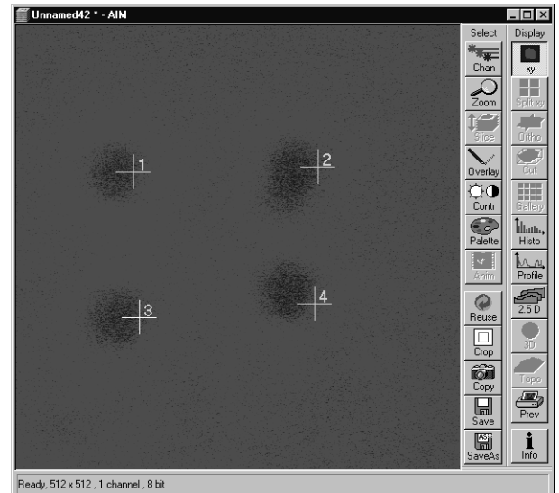
Fig. 4-94 LSM image of the Rh6G layer after bleaching. Deviations between the markers and the bleached spots are noticeable.
