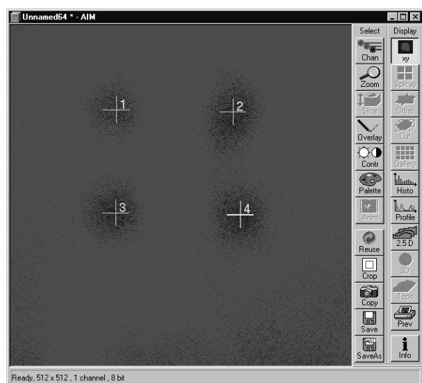
Fig. 4-97 LSM image after bleaching and correction of offset values
