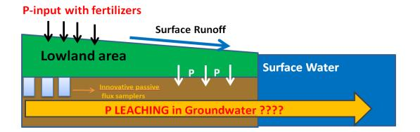
Figure 1: Passive flux samplers to monitor phosphorus fluxes in groundwater
