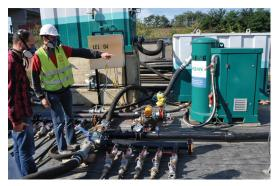
Figure 2. MPE vacuum extracGon pump.
