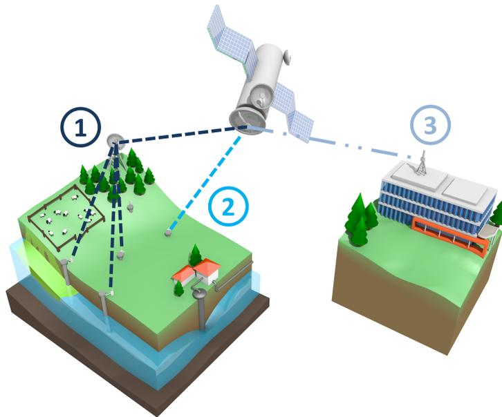
*Figure 4. Conceptual overview of wireless sensor networks, featuring a low-range, node-based (1) and GSM-based (2) setup transmitting data to an off-site server (3).*
