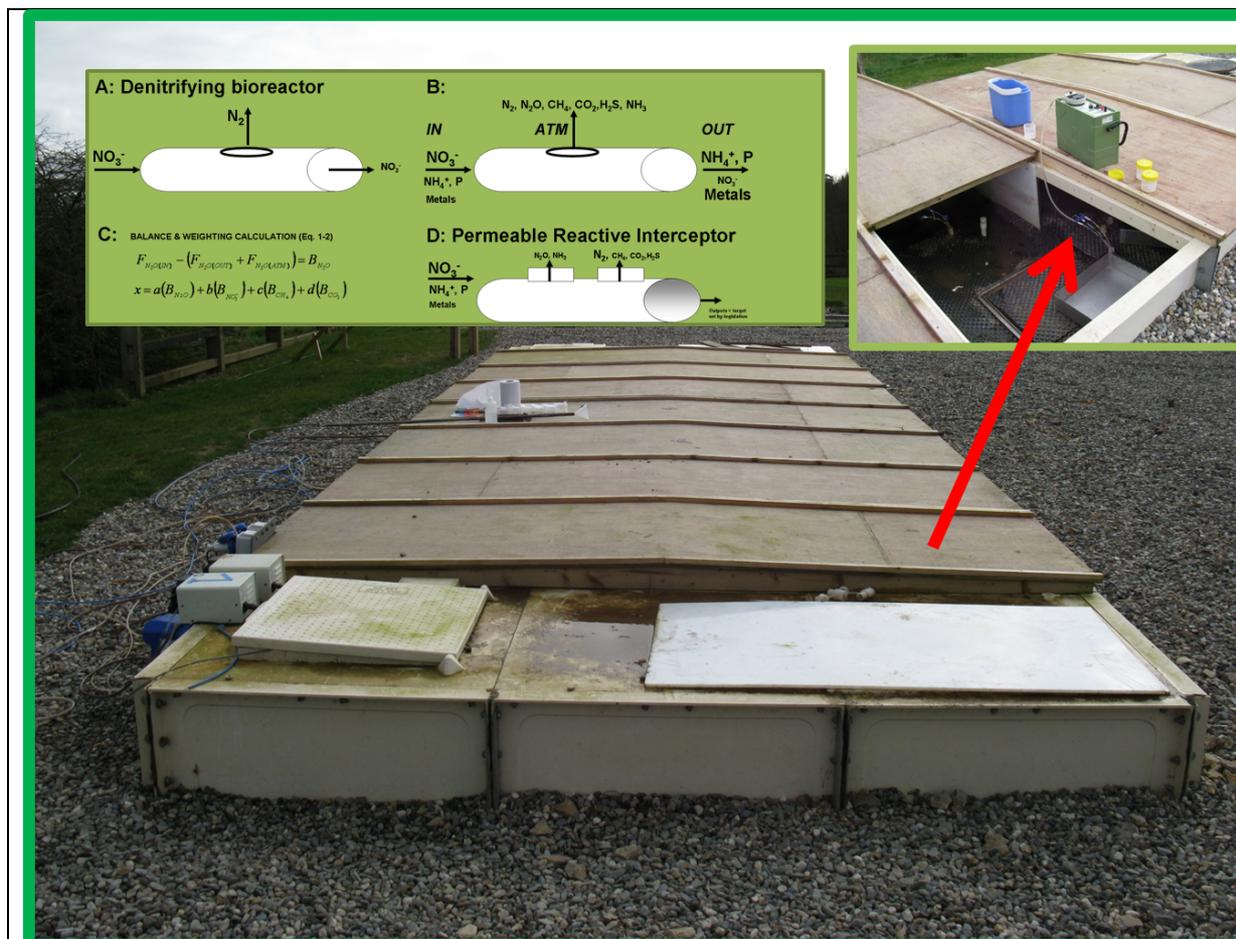
**Figure 7:** The data obtained from the pilot scale denitrifying bioreactor is fed through Eq. 1 and the leaks (if any) in the system are realised. This knowledge can inform the next steps to be taken.
