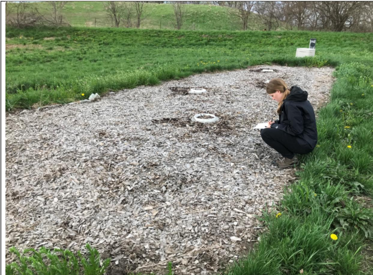
**Figure 6b:** Private farm: Denitrifying woodchip bioreactor in Illinois, USA designed without a soil cover with surface gas emissions sampling chambers shown; Credit: L. Christianson/UIUC and Illinois Farm Bureau.
