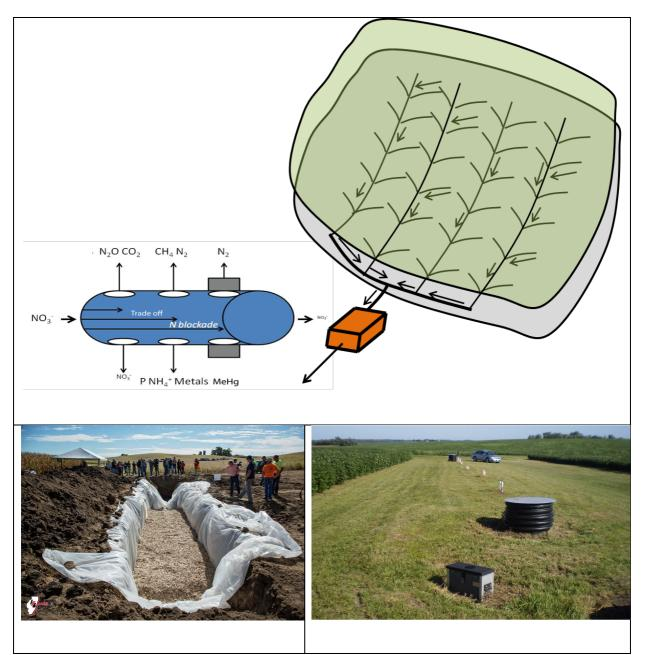
**Figure 1:** Top – concept of the location of a denitrifying bioreactor at the end of a tile drainage system. N blockade – this is a schematic of a leaky pipe which outlines the pollution swapping potential of systems even where N output is less than N input. Bottom – photo of a woodchip filter installation and a soil capped system.
