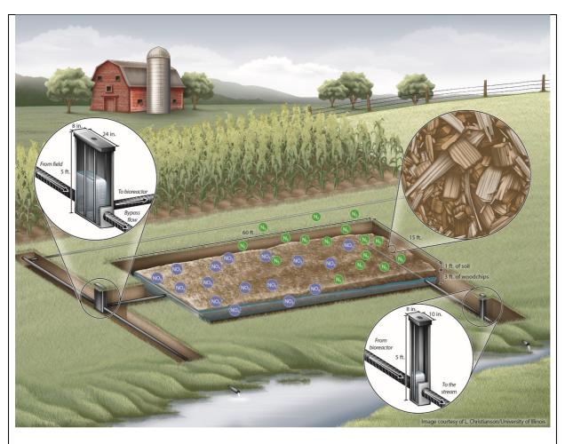
**Figure 8:** Generalized schematic of a denitrifying bioreactor to treat nitrate in subsurface drainage in the US Midwest. Credit: L. Christianson/University of Illinois.
