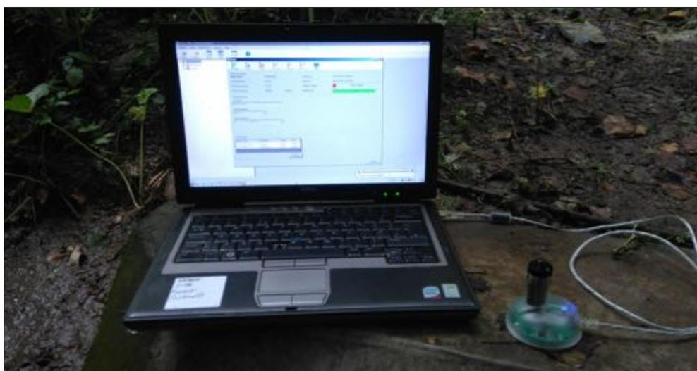
Figure 6. Downloading diver data onsite to elucidate the height of water flowing through the weir. This helps with calculating the load of nutrients flowing through the weir throughout the year.
