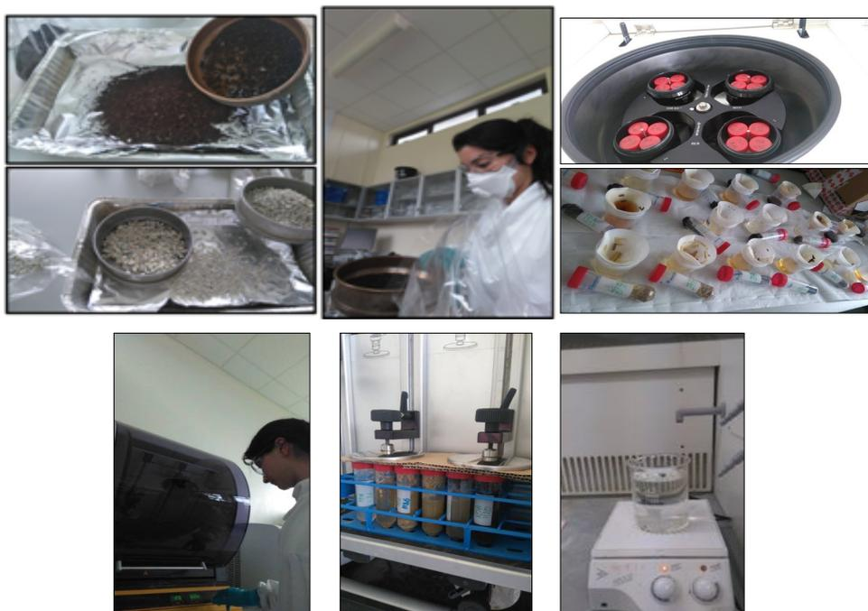
Figure 11. Adsorption test: media preparation, sieving, solution preparation, shaking, centrifuging, filtering
