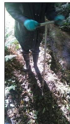
Figure 10. Bankside soil sampling (left) and augering (right)
