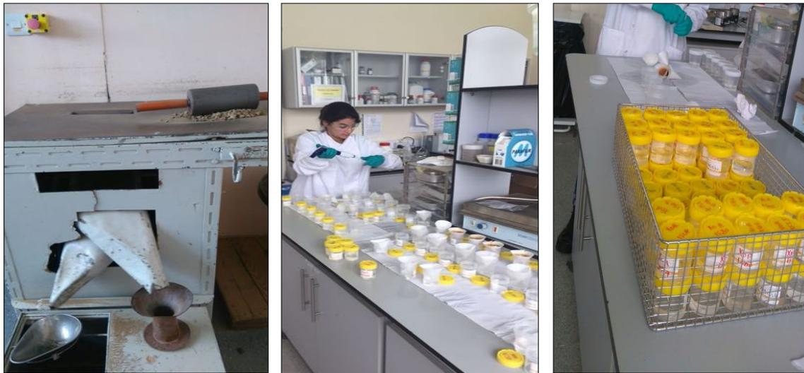
Figure 12 Automatic soil sieving machine (left); Phosphorus isotherm extraction (middle and right)
