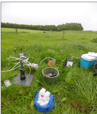
Figure 3. Water sampling equipment: Peristaltic Pumps, Tubing, Battery, *In situ* Probe, Dipper (groundwater depth measuring tool)
