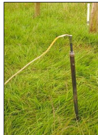
Figure 7. soil gas sampling using an air lance
