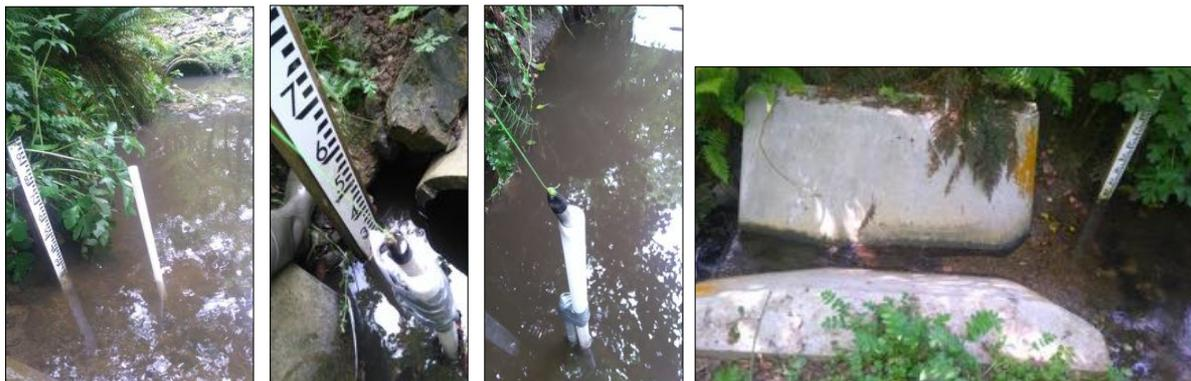
Figure 5. Installation of divers into piezometer in front of a weir
