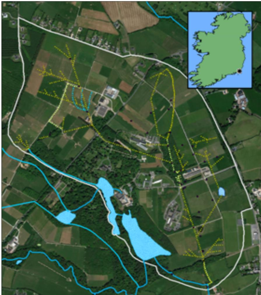
**Figure 2.** Johnstown Castle Mini-Catchment boundary in SE Ireland. Artificial lakes are shown in blue. Green dotted lines and light green lines represent subsurface and surface drainage systems, respectively. The black dots across the map show water sampling points e.g. multi-level wells, surface sampling points, and end of pipes.
