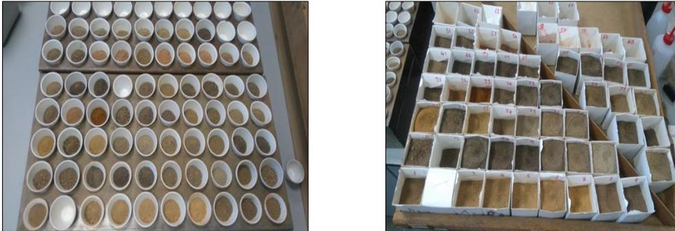
Figure 14. Organic Matter test (left) and soil sample preparation (right)
