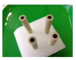
Solid-contact electrodes after carbon nanotubes deposition and before membrane deposition.
