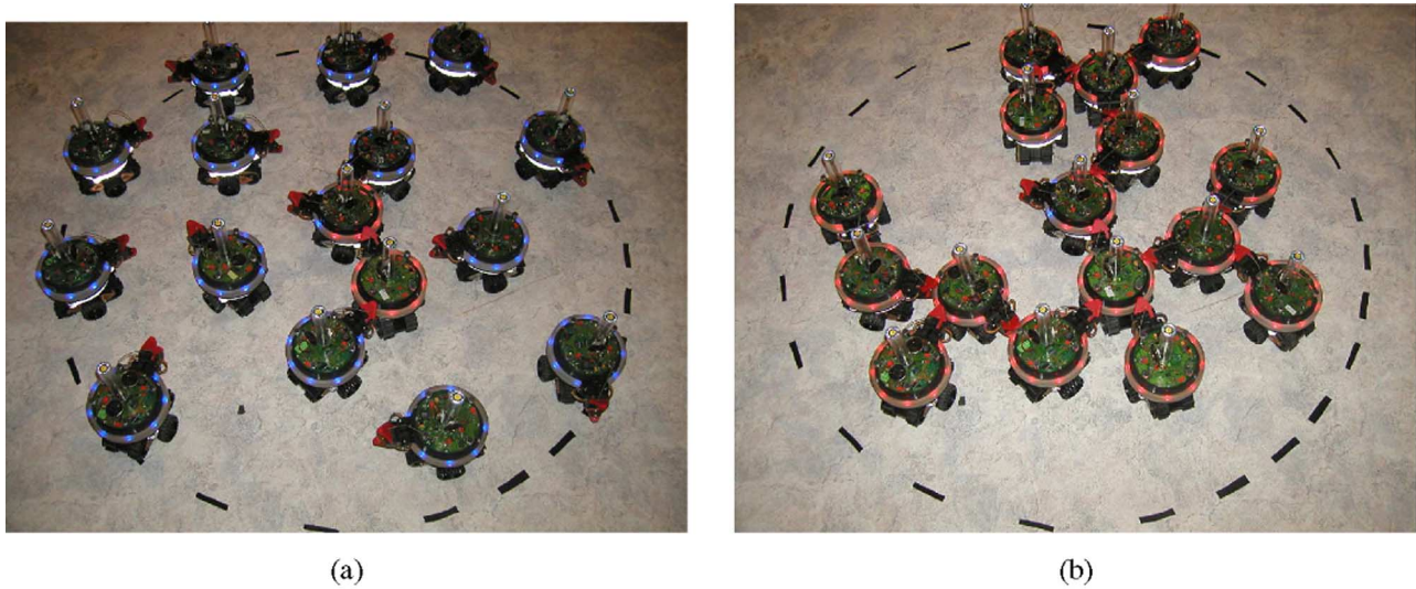
Fig. 20. Self-assembly of 16 physical s-bots put in a circle of radius 50 cm. Trial 12: (a) 19 s and (b) 104 s after activation of the seed.
