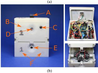
Fig. 7. Prototype module: (a) Assembled module. (b) Internal circuitry in the opened upper section (top right), micropumps in situ in the bottom section (bottom right) and annotated module (left). A: External programming port. B: Magnetic switch (mounted internally). C: The corresponding magnet. D: LDR mounted behind a clear barrier. E: Micropump output port. F: Connection magnets (mounted internally).
