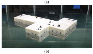
Fig. 1. Modular Hydraulic Propulsion: (a) 3-D simulation of a robot, comprising 512 cubic modules, approaching a target in a fluid environment. Each module can route fluid between any of its faces. By deciding how to route the fluid through the structure, both translation and rotation can be controlled. (b) 2-D physical prototype floating in a water tank. Each module is square shaped and contains four micro-pumps, one per side. When a pump is off, it acts as a bypass.
