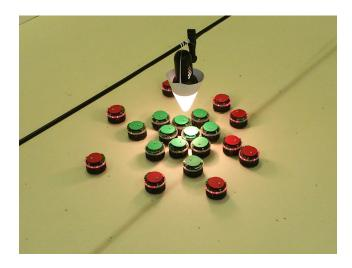
Figure 1: A segregation pattern in a swarm of 20 e-puck robots. The robots have organized into a center-periphery pattern around a light bulb. Robots with green and red top markers emulate disks of radius 8 cm and 16 cm, respectively. Each robot's motion is governed by a combination of three components: (i) attraction towards the light bulb, (ii) random motion, and (iii) repulsion from nearby robots.
