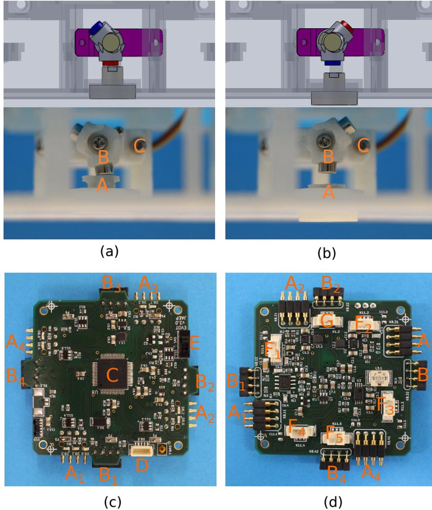
**Fig. 3** (a-b) The anchor mechanism (CAD and real) showing the anchor magnet (A), the rotatable magnet (B), and the servo (C). The anchor is shown in start position (a) and stop position (b). (c-d) The top (c) and bottom (d) layers of the PCB, showing the spring-loaded connectors ( $A_1$  to  $A_4$ ), the pad connectors ( $B_1$  to  $B_4$ ), the microprocessor (C), the programming port (D), the on/off switch (E), the servo connectors ( $F_1$  to  $F_5$ ), and the battery connector (G).
