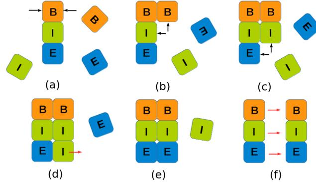
**Fig. 1** Process by which an organism builds a replica of itself. (a) The organism’s *b*-module activates its connectors; (b) and (c) two matching modules connect to the organism; (d) a non-matching module connects but is rejected; (e) a matching module connects; the child organism is complete and receives energy from the parent organism; (f) the parent organism repels the child organism.
