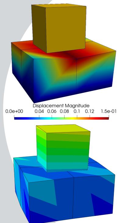
Figure 2. The visualised displacement magnitude from the MATLAB model (above) and the Abaqus model (below). The legend applied to both models.
