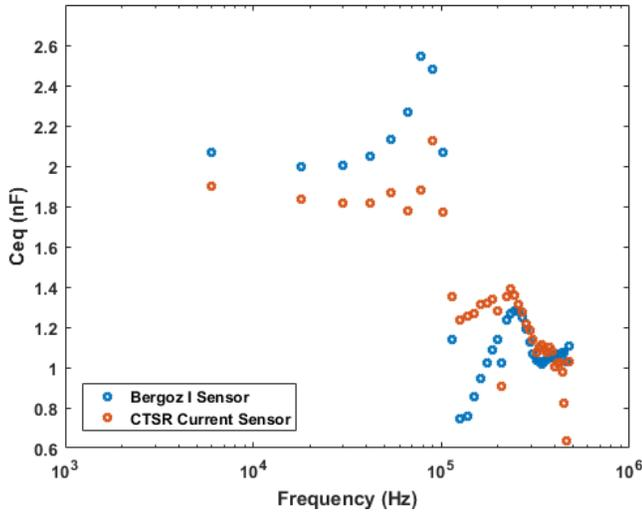
Fig. 9. Capacitance Measurement Comparison CAS Sensor and reference Bergoz sensor.
