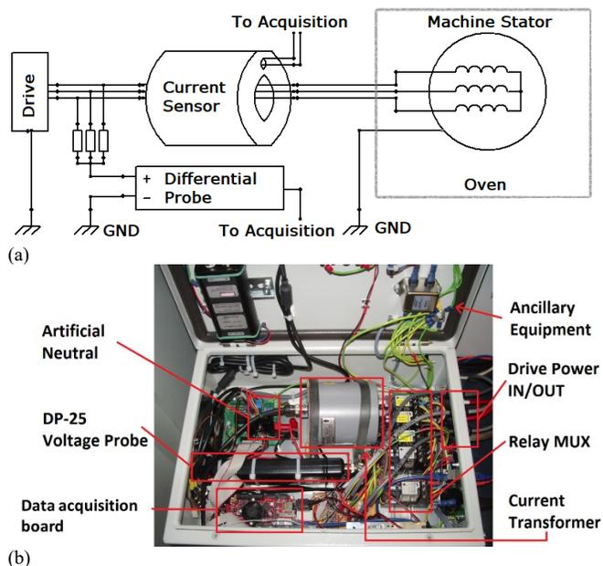
Fig. 3. Block diagram (a) and photo (b) of the experimental rig for the reference design of the CM impedance measurement systems
