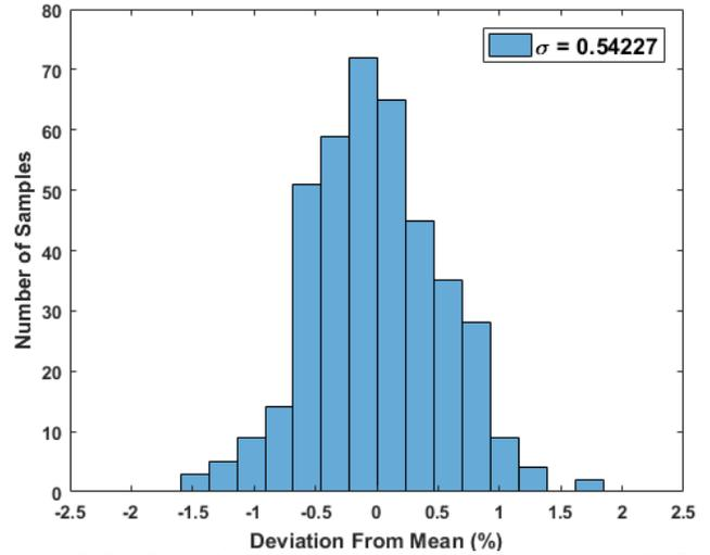
Fig. 10. CM Capacitance at 6kHz measurement deviation for CAS Sensor
