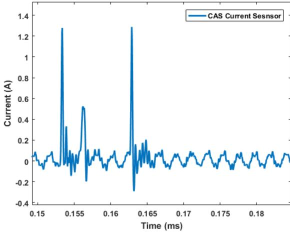
Fig. 8. CM current measurement with CAS sensor
