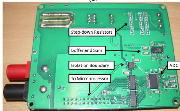
Fig. 4. Schematic (a) and photo (b) of the isolated CM voltage sampling circuit
