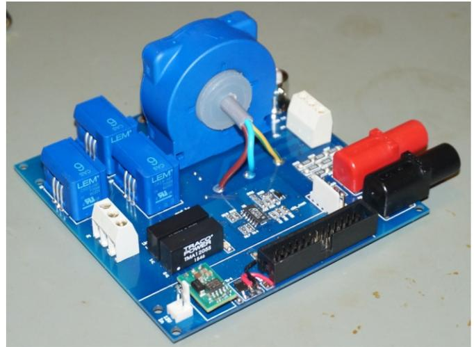
Fig. 12. CTSR Current Sensor System
