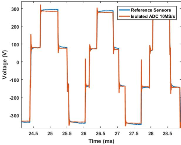
Fig. 5. CM voltage measurement with reference differential probe and proposed circuit
