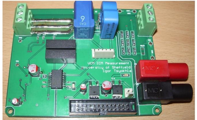
Fig. 7 CM current sensor circuit
