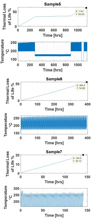
Fig. 5 Thermal cycling experimental results for Samples 2 to 7: samples' temperatures and thermal loss of life
