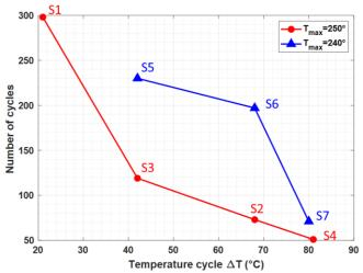
Fig. 8. Number of cycle to failure for the 7 samples as a function of temperature cycling and maximum temperature.
