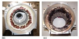
Fig. 2 Machine sample (a), prior to ageing (b) and after failure (c)
