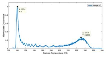
Fig. 3 Hystogram of temperature distribution for sample 7 during its lifetime
