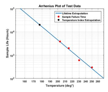
Fig. 4: Lifetime as function of temperature for 4 samples at constant temperature
