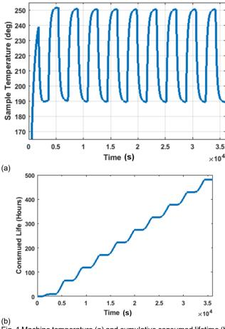
Fig. 1 Machine temperature (a) and cumulative consumed lifetime (b)
