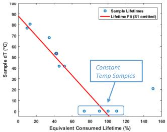
Fig. 6 Consumed lifetime at the time of failure as function of  $\Delta T$
