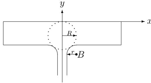
Point  $B$  ( $t_w/2 + r, -t_f - r$ ) lies, not on the circle described by (1), but on the slightly larger circle with the same centre, and radius  $R + r$ . The equation of this circle is
