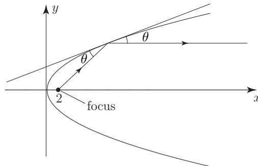
If your sketch is sufficiently accurate you should find that light-rays (lines) parallel to the  $x$ -axis when reflected off the parabolic surface pass through the focus. (Draw a tangent at the point of reflection and ensure that the angle of incidence ( $\theta$  say) is the same as the angle of reflection.)
