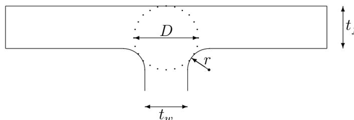
As  $D$  occurs in the form  $D^4$ , the torsion constant is very sensitive to it. Calculation of  $D$  is therefore a crucial part of the calculation of  $J$ .
