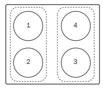
If the right and left cooking zones of hob operates at the same time, the cooking zones operate discontinuously. Therefore the cooking and pan detection performance decrease.
