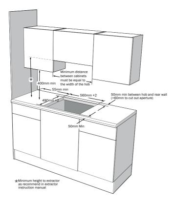
No shelf or overhang of combustible material should be closer than 650mm directly above the hob. There must be a minimum clearance of 50mm between the rear edge of the hob and the rear wall. This clearance must be maintained up to 650mm above the worktop (unless otherwise stated in your extractor manual).
