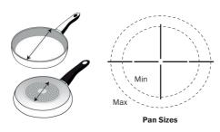
Modern pans are often made using alloys of different materials such as aluminium or copper (Non-ferromagnetic) but use a steel disc in their base to make them compatible with induction hobs. The diameter of this disc may be smaller than the actual pan base and it may also be quite thin. These factors can lead to reduced performance or problems of pan detection.
