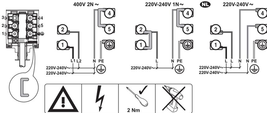
**i** Insert the shunts
