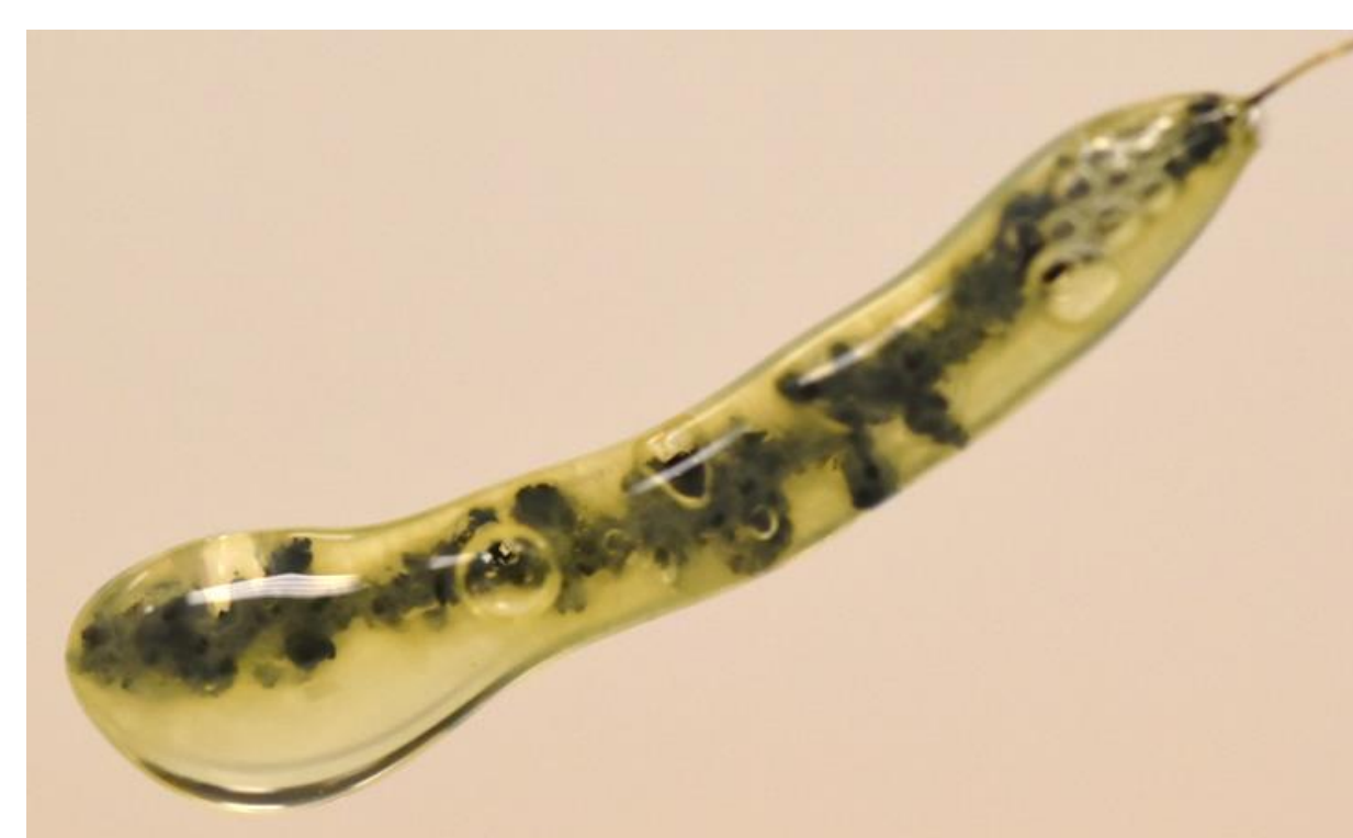
Fig. 5 Photo of PEDOT Chitosan hydrogel sample.
