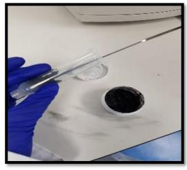
b. *3D printing strain sensors on the glove* (Method used: extrusion)
