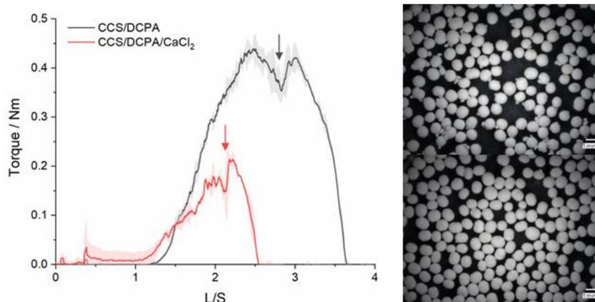
Figure 1. Mixer torque rheometry measurements of the two different mixtures (left) and the resulting pellets (top: CCS/DCPA (50:50), bottom: CCS/DCPA/ $\text{CaCl}_2$  (50:43:7)) at the optimal L/S (right)
