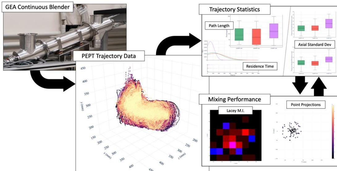
Figure 1. Pipeline showcasing the PEPT experiment and the subsequent analysis.
