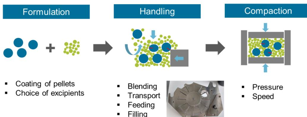
Figure 1. Illustration of influences on pellet coating integrity over a typical tableting process chain
