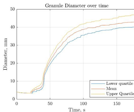
Figure 1. Granule growth behaviour within the DEM simulation, demonstrating induction growth and the distribution of sizes.
