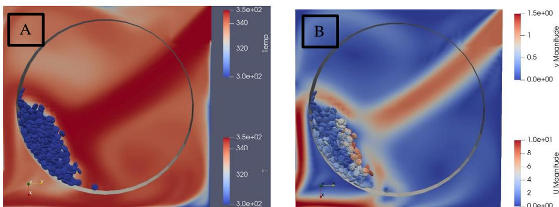
Figure 1. (A) Temperature profile of Tablets (T) and air (Temp). (B): Velocity plot of tablets (v) and air (U)
