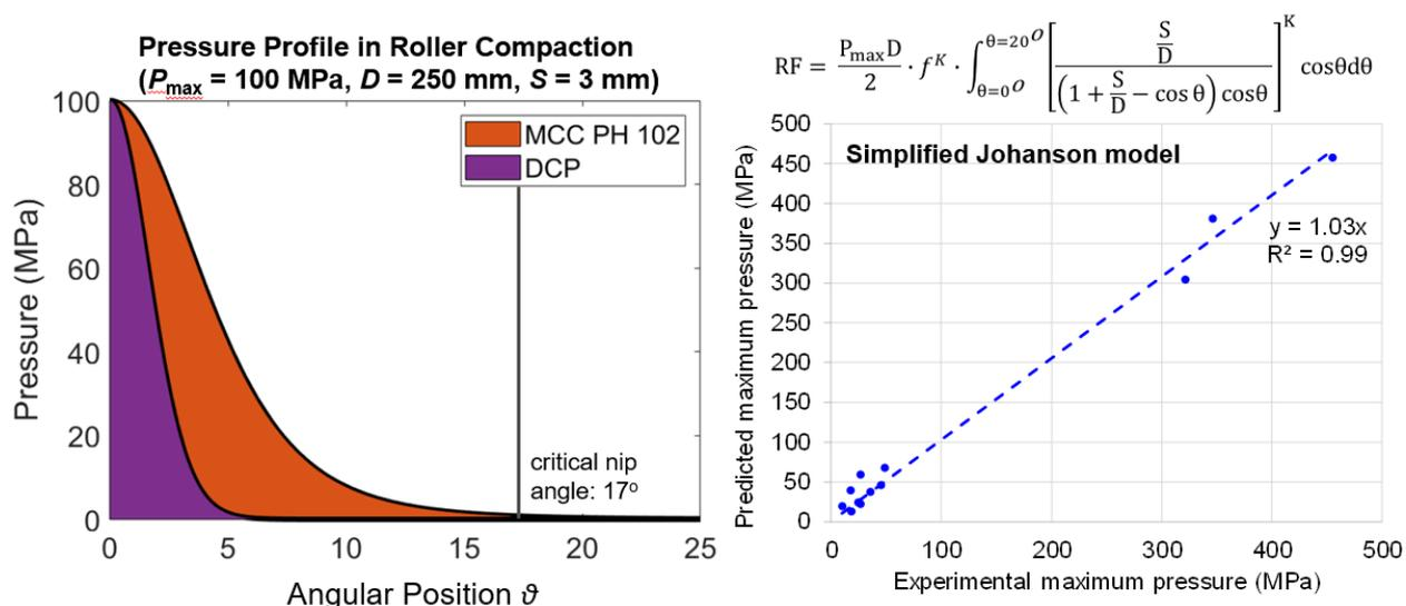
Figure 1. Pressure profile of microcrystalline cellulose and dicalcium phosphate in roller compaction (left), and the experimental  $P_{max}$  vs predicted  $P_{max}$  using the simplified Johanson model (right).
