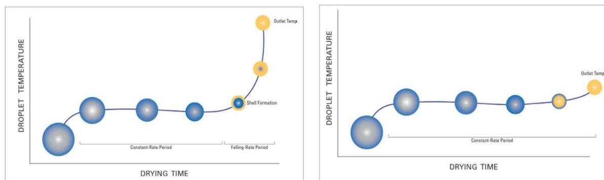
Figure 1. Drying curve of droplet temperature in conventional spray drying and electrostatic spray drying
