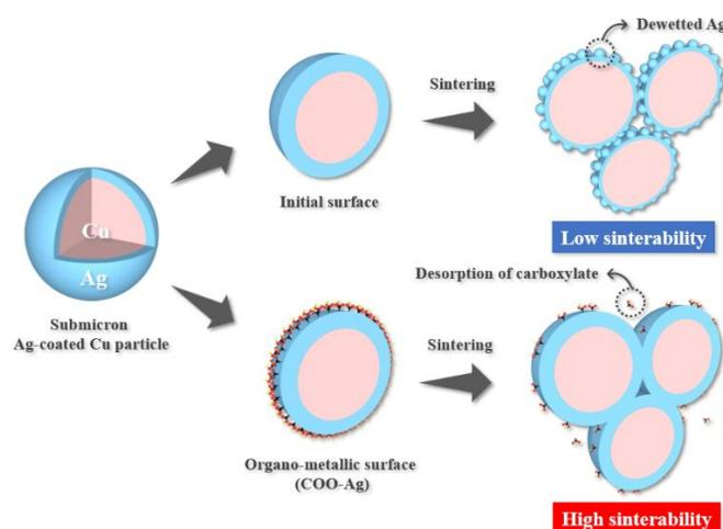
Figure 1. Schematic illustration of different sintering methods using submicron Ag-coated Cu particles
