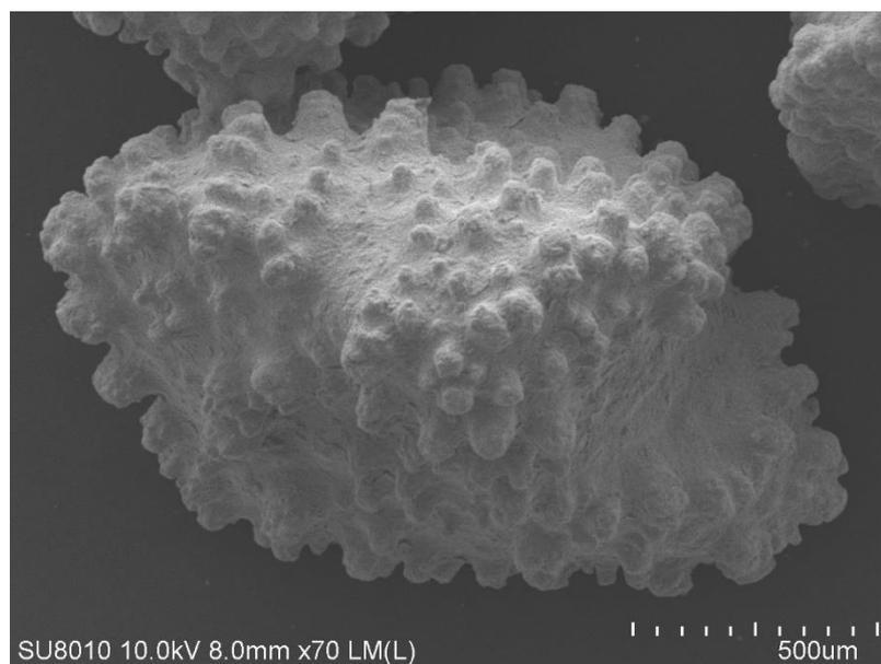
Figure 1. Recovery particle as zinc sulfide using fluidized bed homogeneous crystallization
