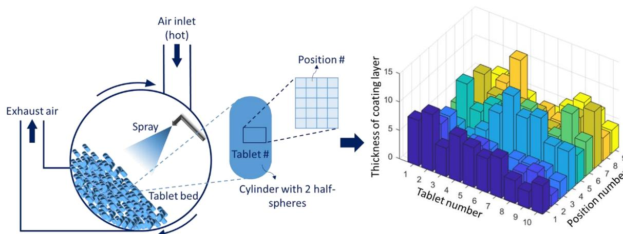
Figure 1. A schematic diagram for analyzing the tablet coating thickness.
