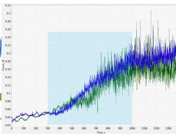
Figure 2. Force measurement during granulation
