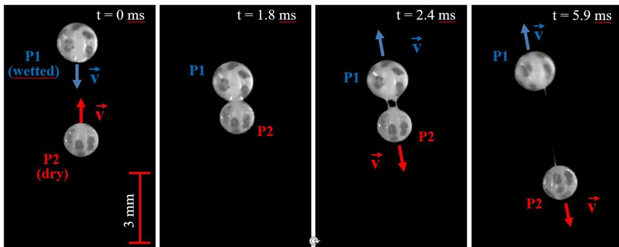
Figure 1. Wetted binary particle collision between two spherical  $\text{ZrO}_2$  particles with a diameter of 1.5 mm. The upper particle (P1) is wetted with a 116.3  $\mu\text{m}$  thick layer of silicon oil with a kinematic viscosity of  $150 \cdot 10^{-6} \text{ m}^2/\text{s}$  at  $20^\circ\text{C}$ , while the lower particle (P2) is dry.
