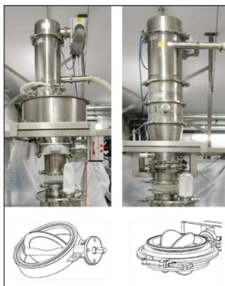
Figure 1. Refillers: TT-refiller (left), G-refiller (right).
