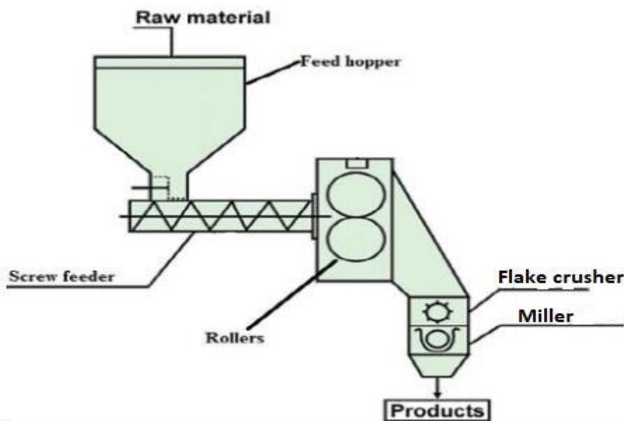
Figure 1. Diagram shows the main parts of roller compactor machine [2]
