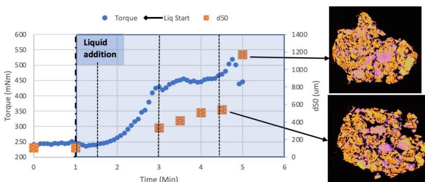
Figure 1. Dynamic median diameter overlaid with torque profile and microstructure images
