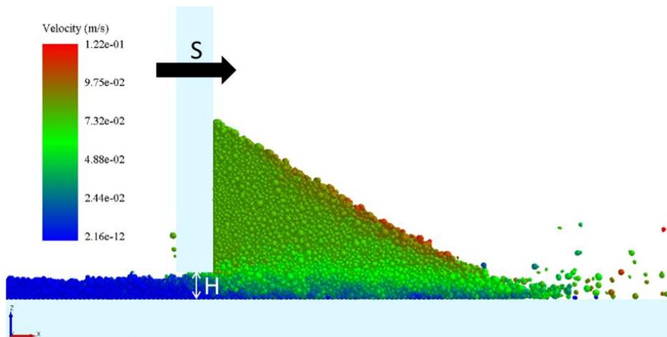
Figure 1. Illustration of powder spreading in EDEM
