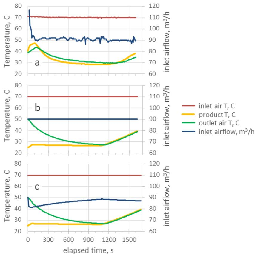
Figure 1. Fluidized bed granulation: a) Process data, Syntegon SolidLab2; b) Feed-forward mass and energy balance at fixed airflow; c) Feed-forward mass and energy balance with integrated fluidization model.
