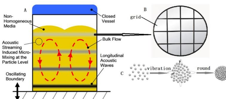
Figure 1. Particle agglomeration with resonant acoustic mixer, A represent the resonant acoustic mixer, B is the grid in the mixer, C shows the brief process of particle agglomeration [2]
