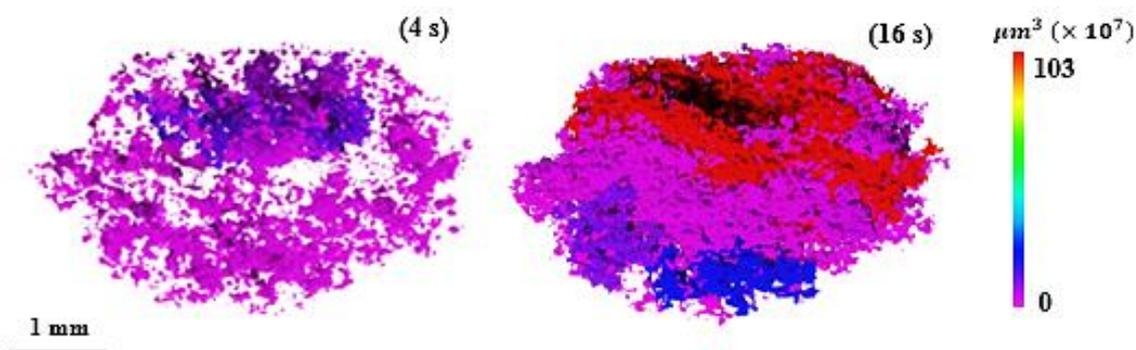
Figure 1. 3D pores volume rendering over time for 50%MCC-50%APAP.
