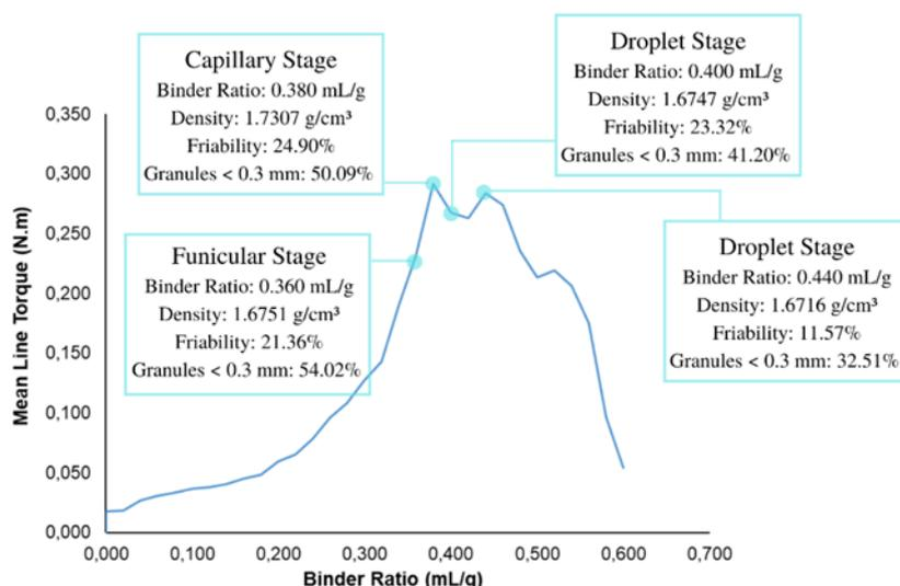
Figure 1. Rheological profile and granule characterization results for different binder ratios.
