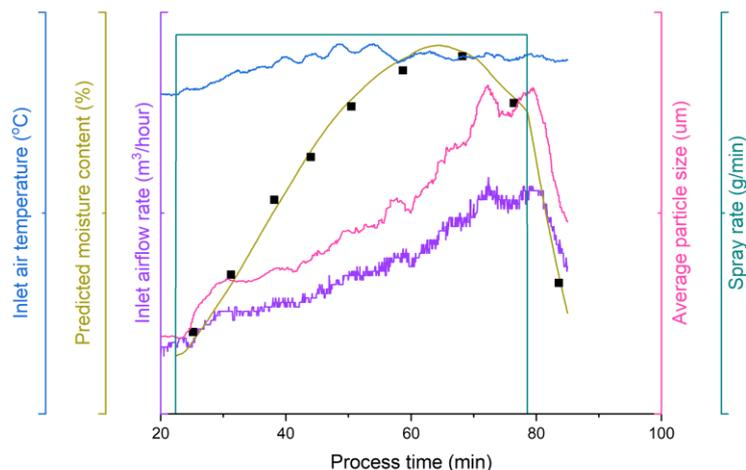
Figure 1. Real time prediction of powder bed moisture content and dynamic control of fluidisation air flow rate during fluidised bed granulation. Black points represent the measured moisture content
