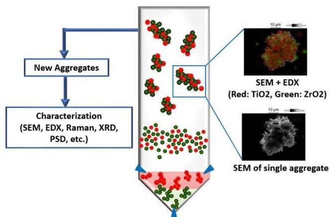
Figure 1. Experimental setup of the opposed-jet fluidized bed.
