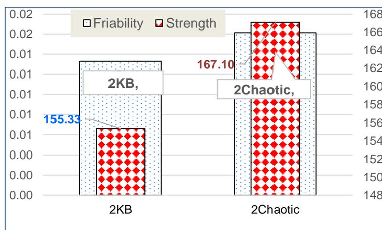
Figure 1. Comparison of mixing elements for tablet friability and strength
