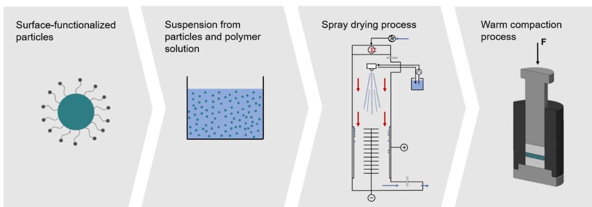
Figure 1. Process route for the production of composite pellets using functionalized particles by spray drying and warm compaction.
