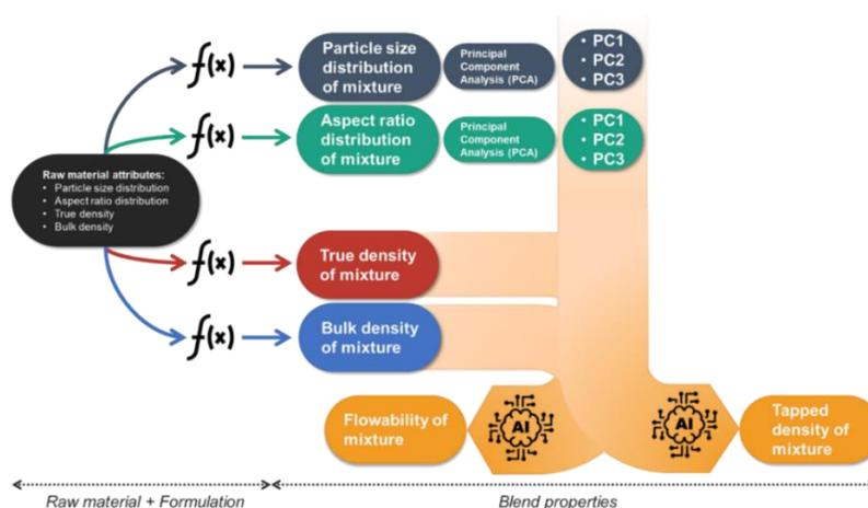
Figure 1 - Flow diagram of the proposed hybrid framework for mixture modelling.  $f(x)$  and AI represent mechanistic and data-driven models, respectively.
