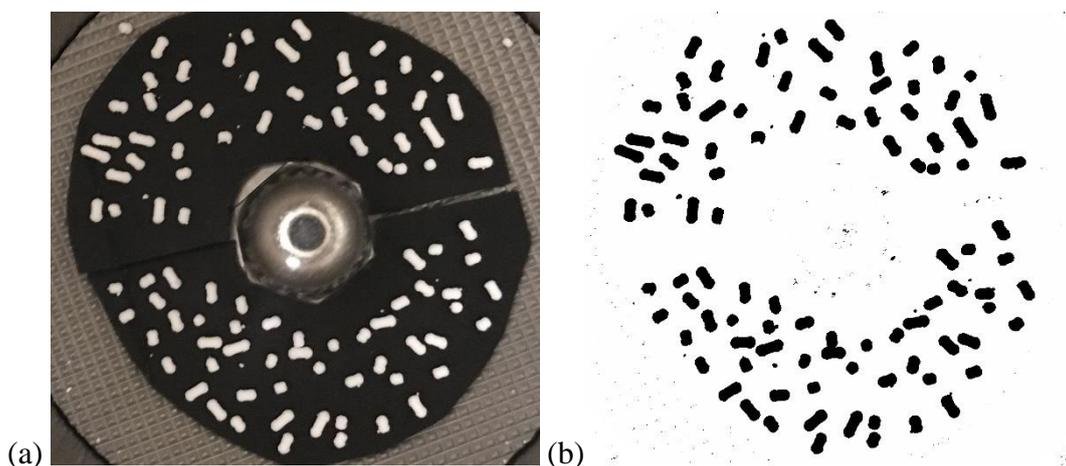
Figure 1. Photograph (a) and binarised image (b) used for shape analysis
