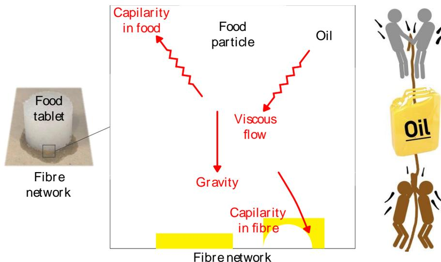
Figure 1. Schematic of different drive and resistance processes occurring during oil-release from particle food systems to fibre-based packaging, in analogy to a tug competition for oil.
