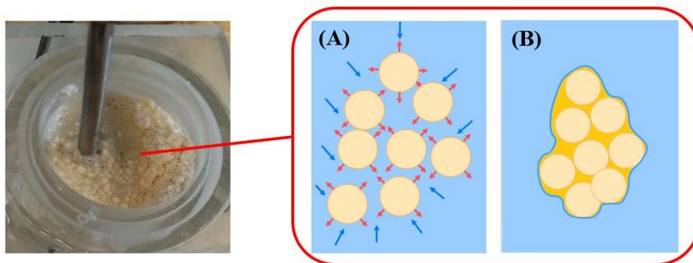
Figure 1. Lump formation during reconstitution, (A) particles start to swell (red arrows) due to water contact (blue arrows); (B) formation of a viscous outer layer leading to the aggregation of swelling particles
