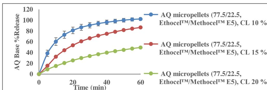
Figure 1. Percentage of AQ released from 77.5/22.5 (Ethocel™/Methocel™ E5) coated micropellets at different coating levels versus time (minutes).
