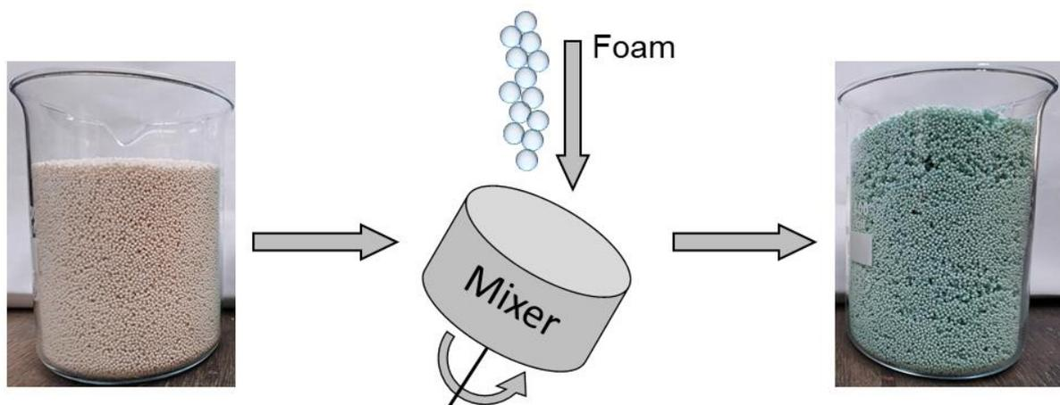
Figure 1. Foam coating of cellulose pellets
