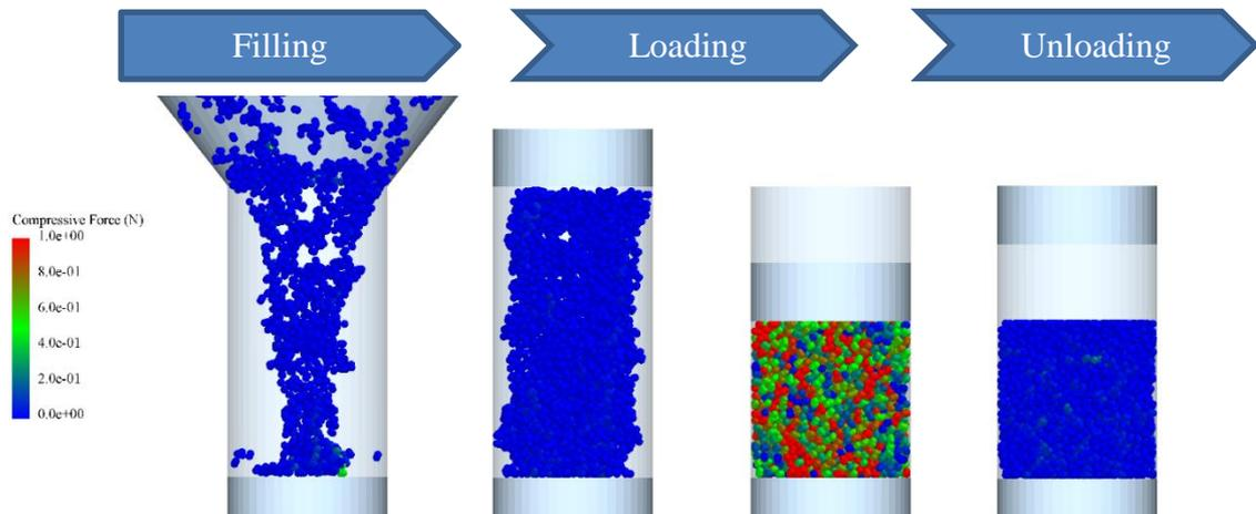
Figure 1. Snapshot of a DEM simulation for particles clipped up to the middle plane in an indie uniaxial compression test, EDEM (Altair Engineering)
