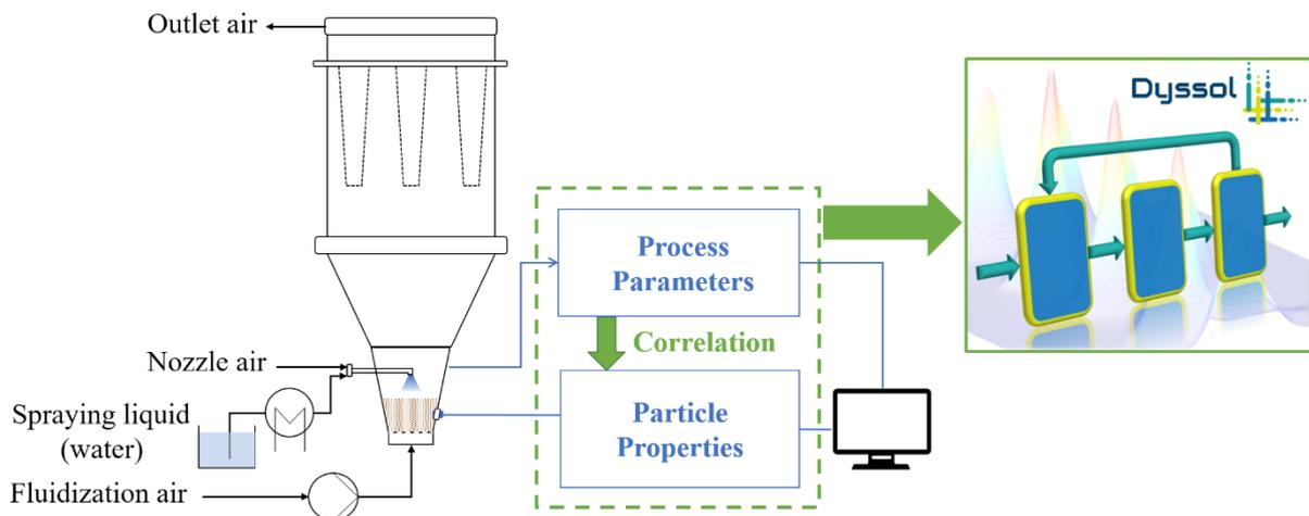
Figure 1. Schematic experimental setup with inline measurement of process parameters and particle properties. The correlation is implemented in the dynamic flowsheet simulation tool Dyssol.
