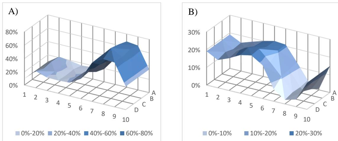
Figure 1. Dependency of different sieve fractions in a PSD on the position under the sieve mill in a roller compactor. A) sieve fraction <0.20 mm, B) sieve fraction 0.40 to 0.63 mm.
