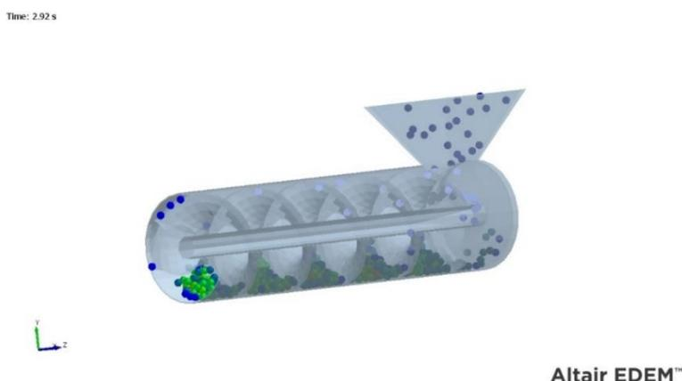
Figure 1. Particle Flow in Variable Density Extruder (VDE)
