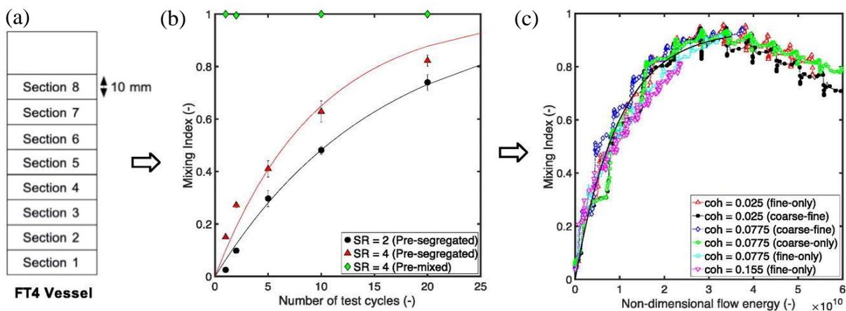
Figure 1. (a) the sectioned FT4 vessel used to assess mixing index (b) influence of particle size ratio on mixing rate (c) the developed relationship to predict mixing rate (black line) mapped against systems of varying cohesion
