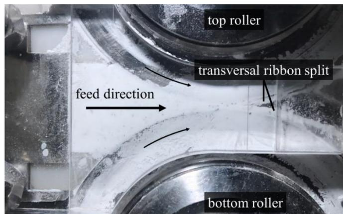
Figure 1. Insides of roller compactor WP120 by Alexanderwerk AG during production with smooth roller surface.
