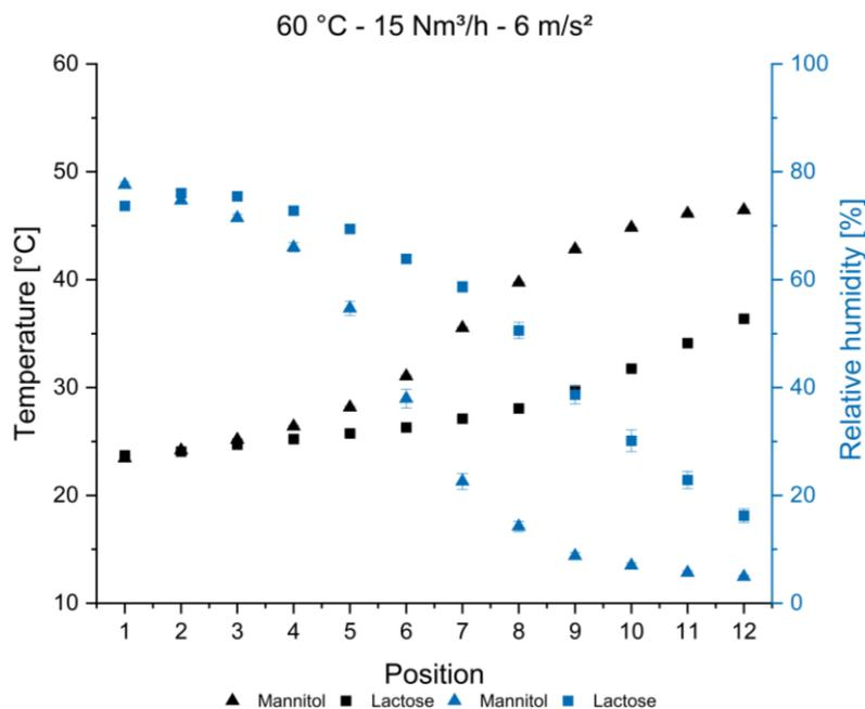
Figure 1. Temperature- and humidity profiles of lactose and mannitol formulation along the drying chamber of QbCon® 1.
