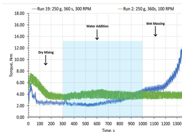
Figure 1. Torque measurement during granulation
