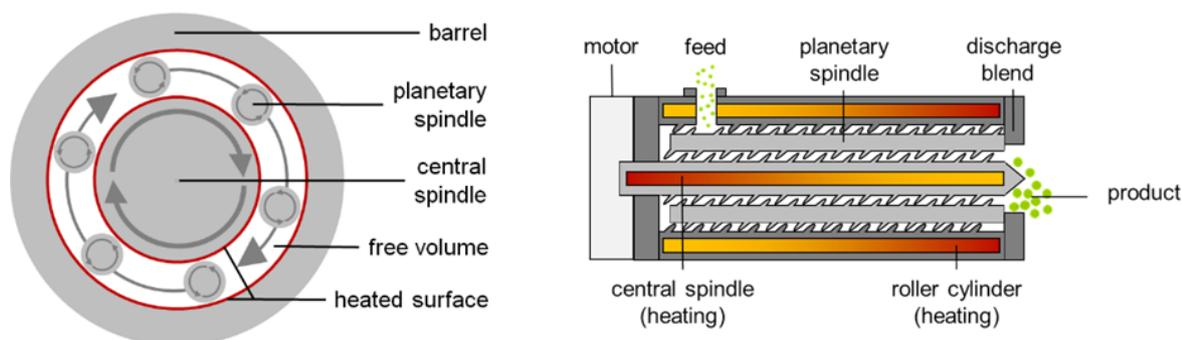
Figure 1. Radial cross section of a planetary roller granulator (left) and axial cross section of the modular machine concept (right)
