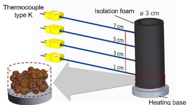
Figure 1. Experimental set up for heat transfer via conduction on moist particle bed
