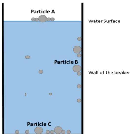
Figure 1. The problem faced when suspending solid particles into liquid. Particle A is floating on the liquid surface. Particle B is sticking on the wall of the beaker. While particle C settles down to the bottom.
