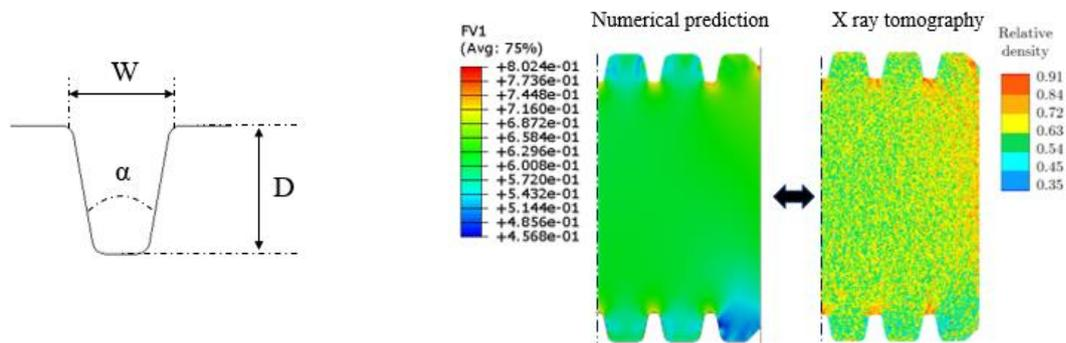
Figure 1. Groove shape (left), relative density distribution of grooved tablet (right)
