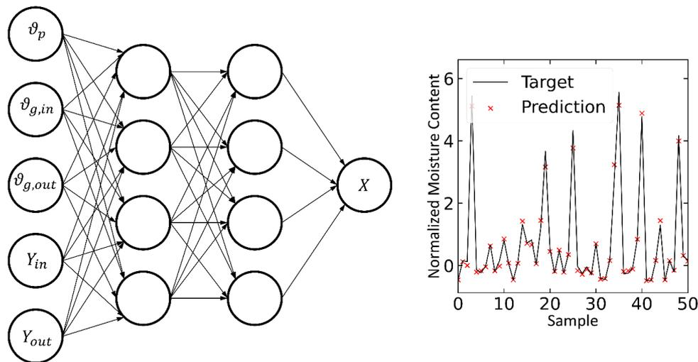
Figure 1. Artificial neural network for the prediction of solid moisture content based on process parameters bed temperature  $\vartheta_p$ , temperature of fluidization and exhaust gas  $\vartheta_{g,in}$  and  $\vartheta_{g,out}$  and moisture content of fluidization and exhaust gas  $Y_{in}$  and  $Y_{out}$ . The topology is shown on the left and a prediction on random samples of a batch drying of Cellets®200 is shown on the right.
