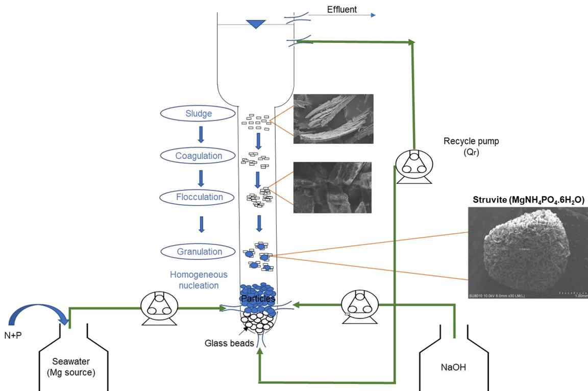
Figure 1. Fluidized bed homogeneous reactor (FBHC) arrangement.
