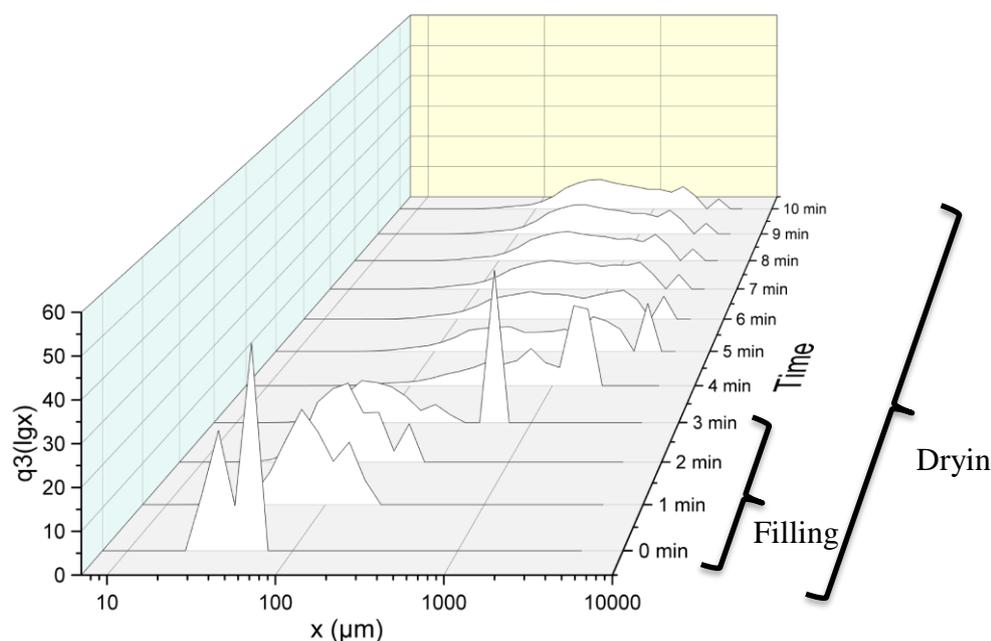
Figure 1. Volume density distribution  $q_3(\lg x)$  with time, filling stage lasts for 3 minutes and total drying time is 10 minutes. 0 minute is defined as the time granules are detected by the probe.
