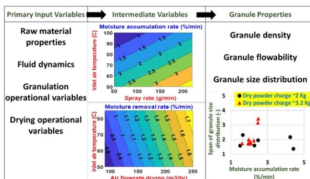
Figure 1. Connecting granulation process inputs with granule properties via intermediate variables
