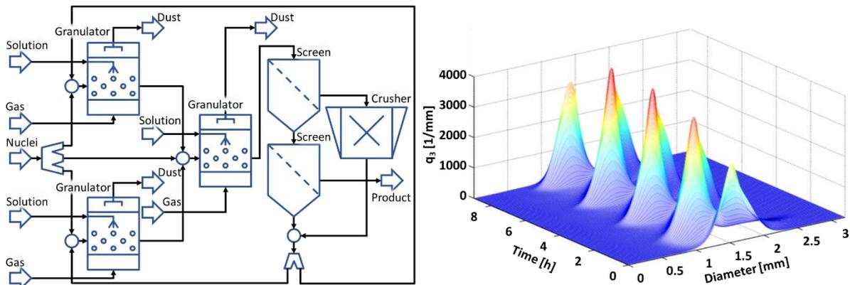
Figure 1. An example flowsheet of a two-stage granulation process with external classification and milling (left) and a time-dependent change in particle size distribution of granules (right).
