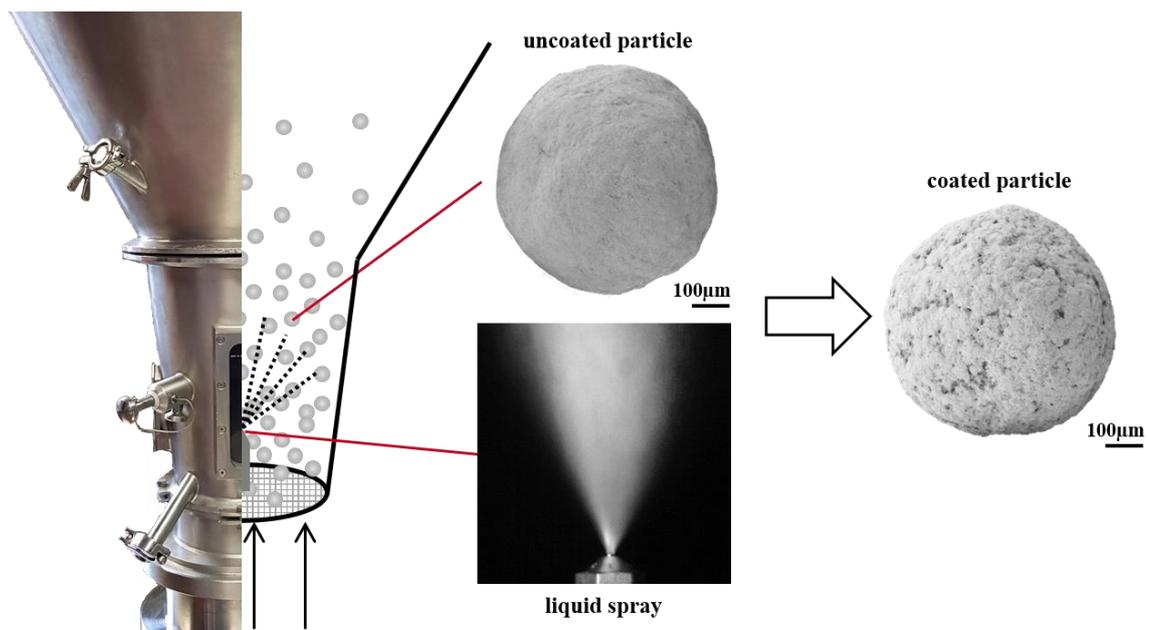
Figure 1. Scheme of a fluidized bed spray granulation with highspeed camera image of the spray cone and SEM images of uncoated and coated particles.
