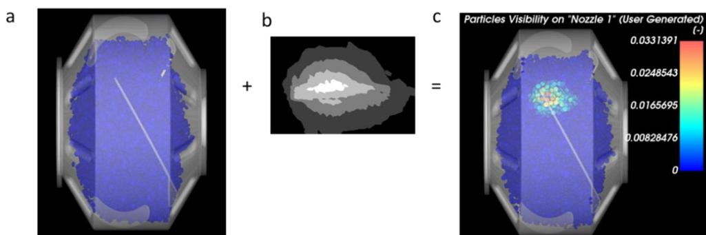
Figure 1. (a) Tablets in a drum coater, (b) spray distribution contour, and (c) snapshot of coated tablets with spray.
