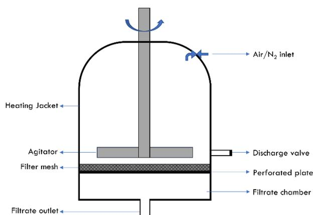
Figure 1. Cross-sectional representation of an AFD.
