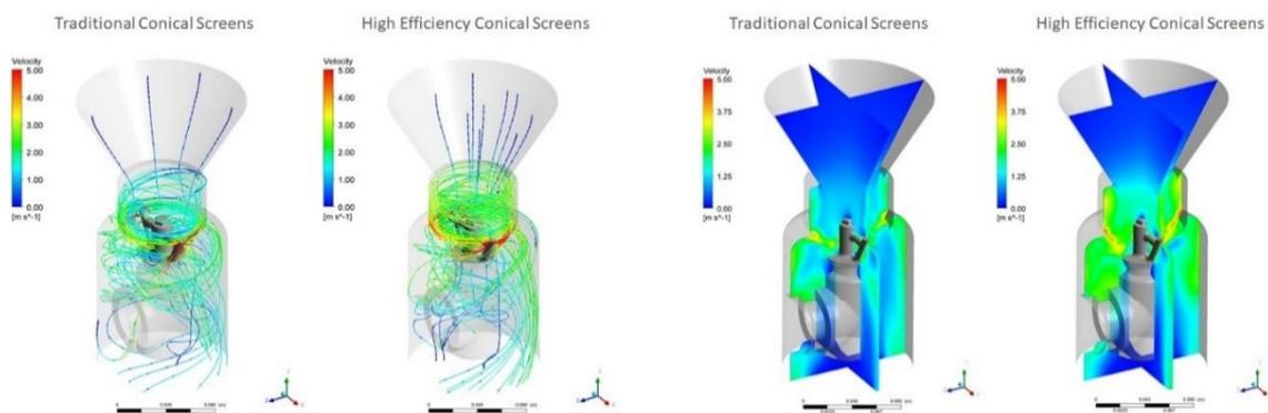
Figure 1. Air Flow (left) and Mass Flow (right) Across Traditional vs. New Hole
