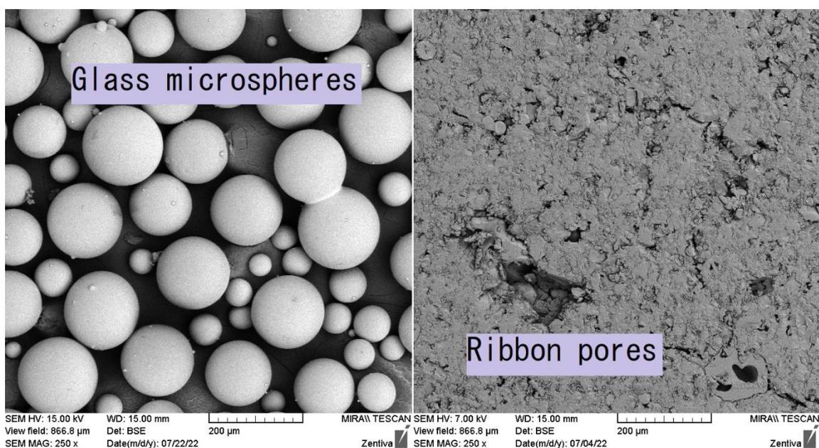
Figure 1. Comparison of glass microsphere size to ribbon pores
