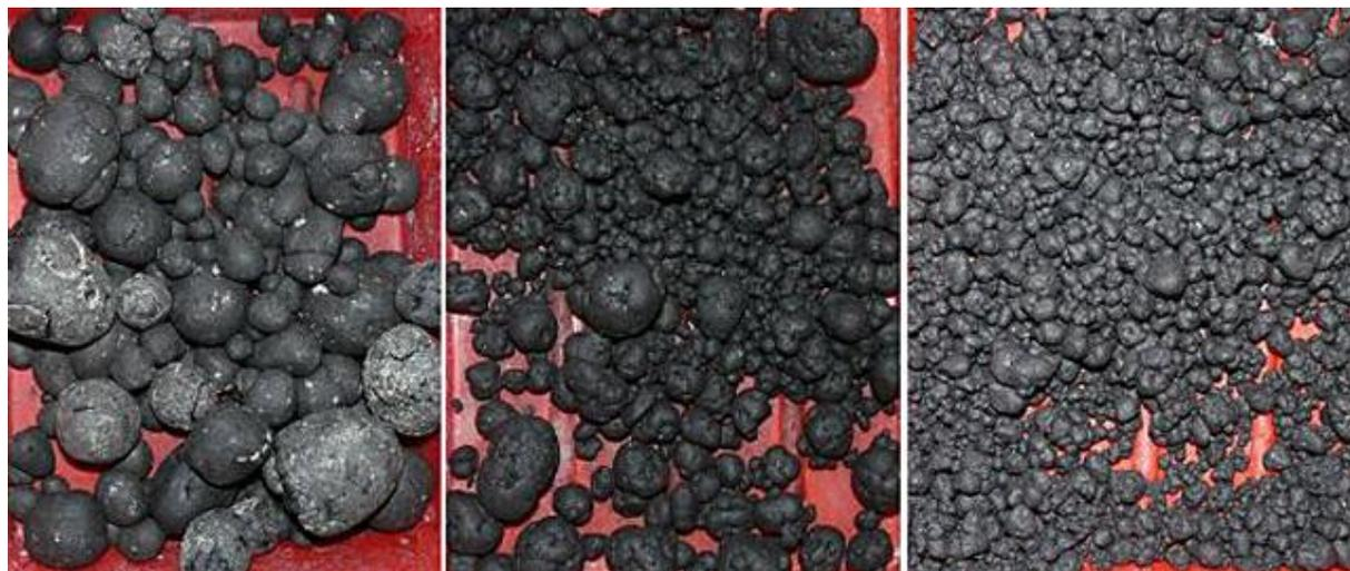
Figure 1. Granules size and shape depending of technological parameters and type of binder
