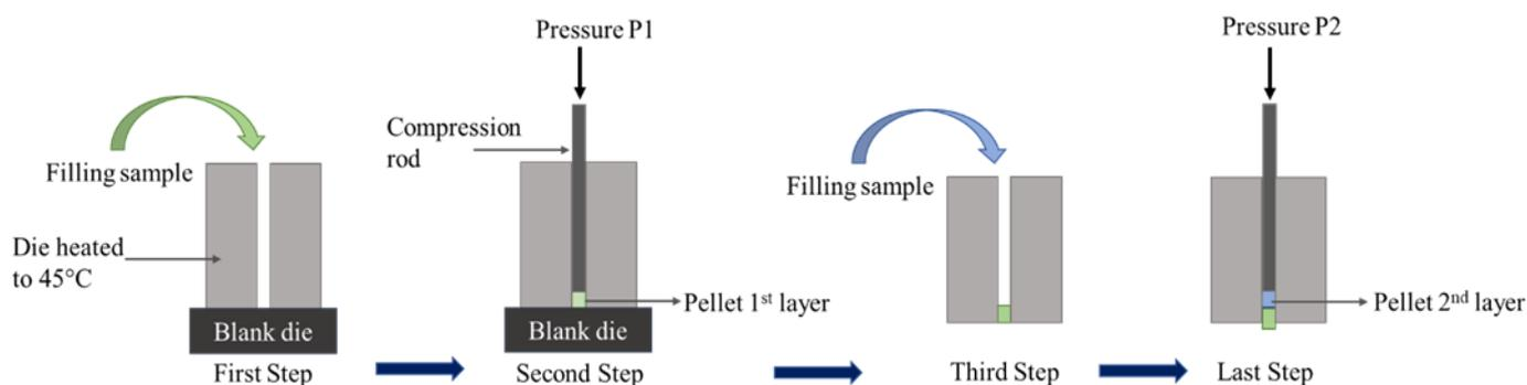
A schematic illustration of the pelleting process using a single-die pellet press.
