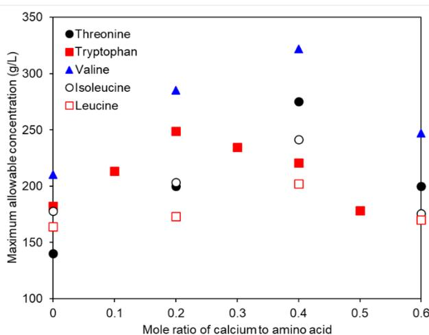
Figure 1. Effect of mole ratio of calcium to amino acid on maximum allowable concentration during the evaporation process of various amino acids
