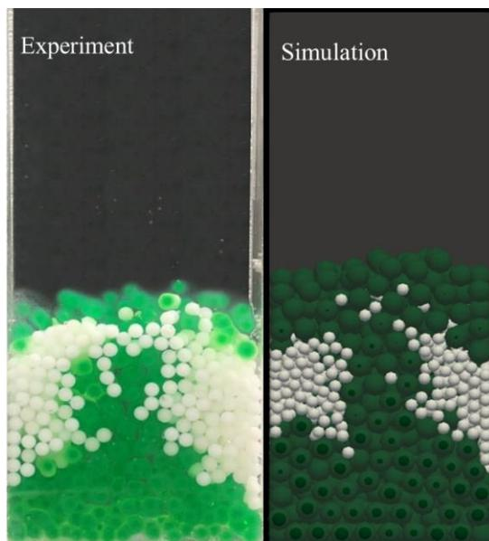
Figure 1. Swelling behaviour of particles in a cubic container
