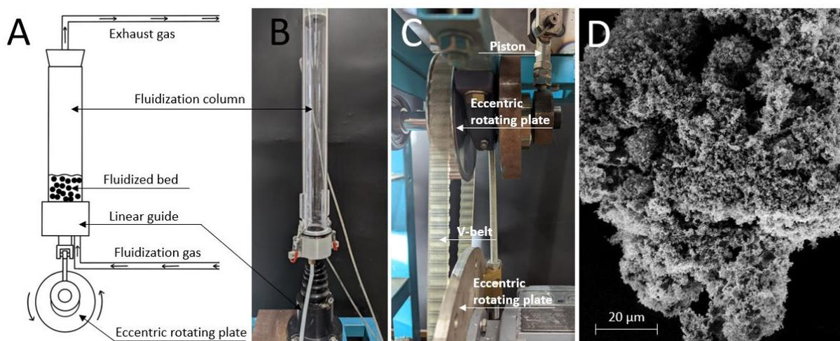
Figure 1. Schematic of a vibrated fluidized bed (A) Upper part of fluidized bed (B) Motorized v-belt system for translation of vibration frequency (C) and an SEM image of LFP coated with CB obtained by fluidization (D).
