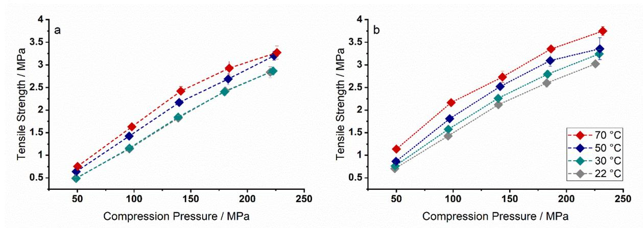
Figure 1. Change in tensile strength for different tableting temperatures. Binary blend containing lactose and (a) HPC SSL (b) HPC SSL-SFP ( $\bar{x} \pm sd$ ,  $n=10$ ).
