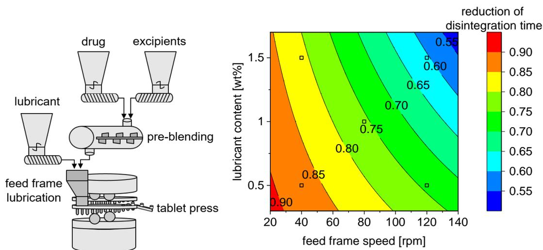
Figure 1. Schematic representation of the feed frame lubrication (left) and contour plot with disintegration time reduction for feed frame speed and lubricant content variations (right).
