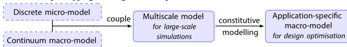
Figure 1. Modeling framework for the virtual prototyping of wet granulation processes
