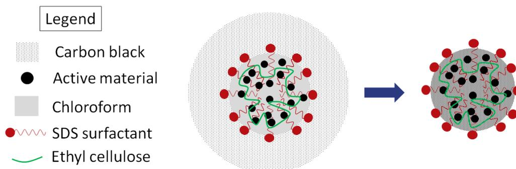
Figure 1. Mechanism of AM-CB co-agglomeration
