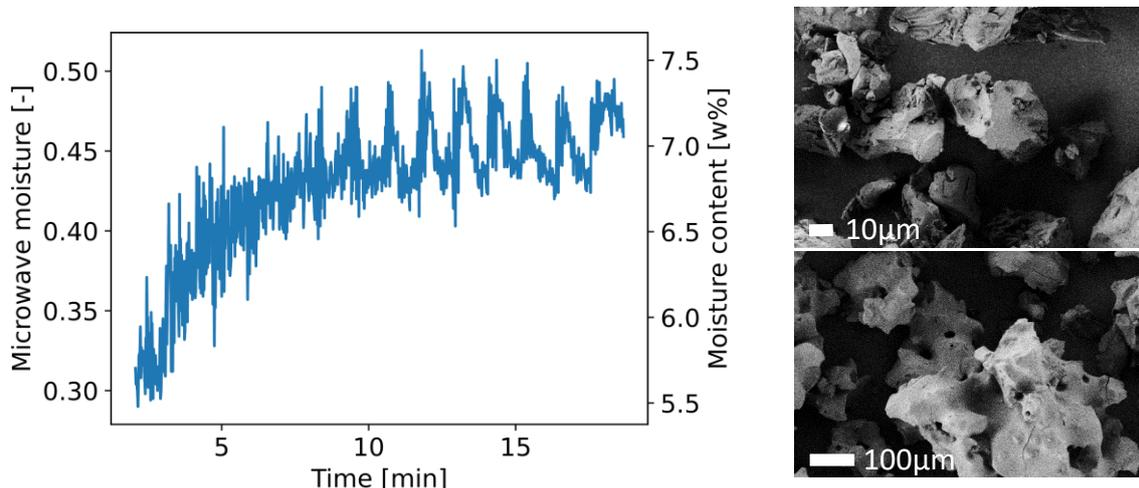
Figure 1. Moisture content over time during batch agglomeration (left), SEM pictures of original maltodextrin particles (right top) and maltodextrin agglomerates (right bottom)
