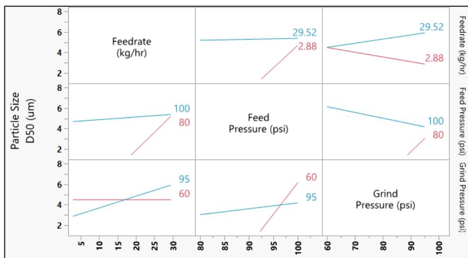
Figure 1. Particle Size D50 vs. Interaction Profiles generated via Fit Model
