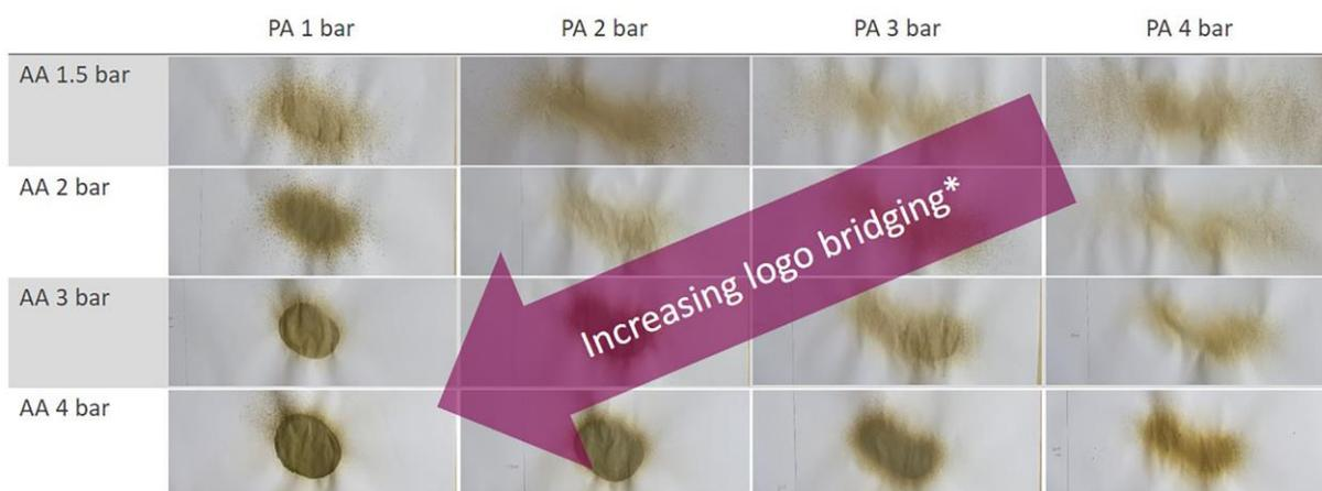
Figure 1. Images of Spray Characterisation with associated Atomization & Pattern air pressures
