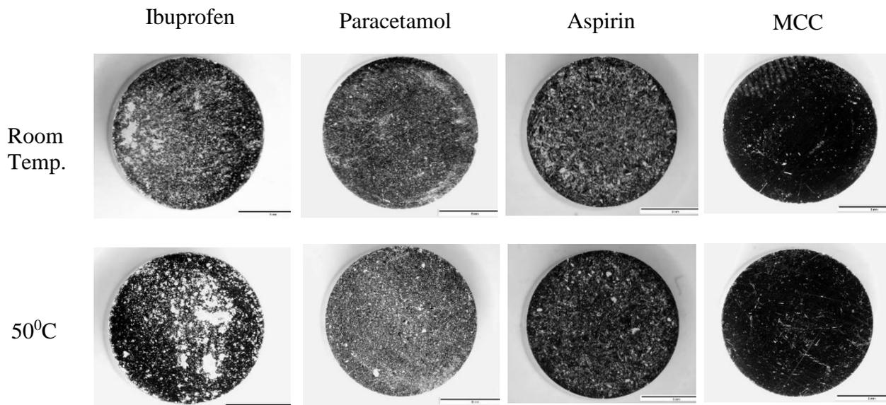
Figure 1. Microscopic images of powder sticking to punch surface at room and elevated temperature.
