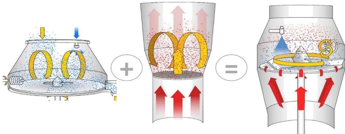
Figure 1. Schematic overview of fusion of traditional high shear granulation and fluidized bed drying into the TwinPro® process.
