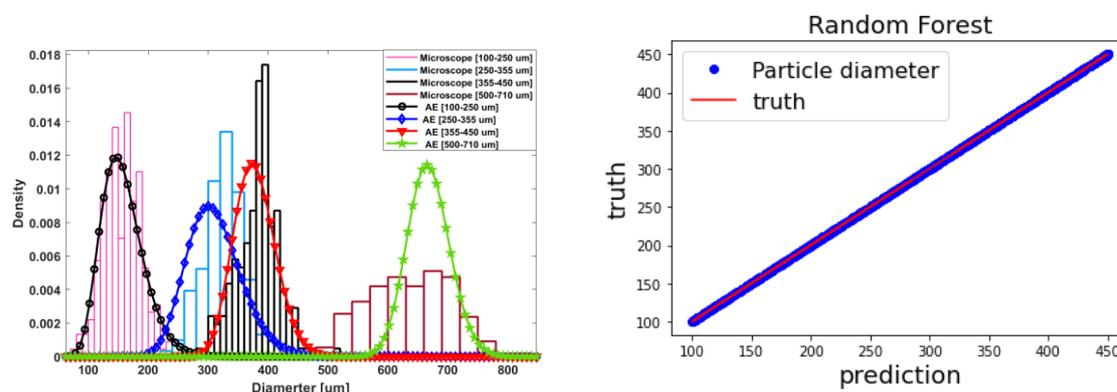
Figure 1. A) Inverted particle size distribution from the measured AE energy, B) Prediction Vs the truth of dataset.
