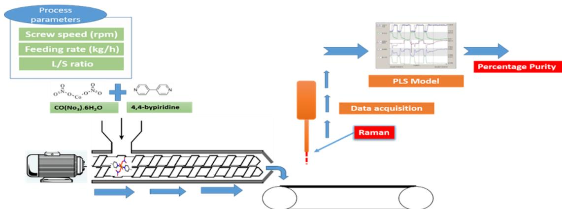
Figure1. Equipment set-up, process parameters and process tools for measuring the purity of the MOF
