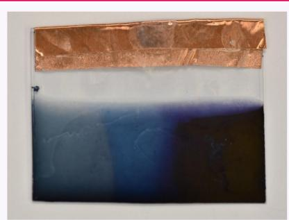
Fig.5 Differential appearance of conductive hydrogels from oxidised and reduced electrodes after bipolar experiment (Light and Dark)
