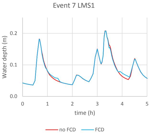
Figure 57 Event 7 water depth simulation with and without FCD at the LMS1
