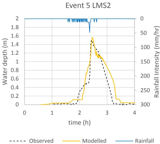
Figure 16 Comparison of water depth observed in LMS2 and modelled
