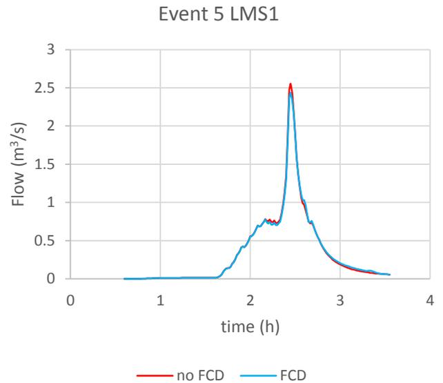
Figure 49 Event 5 flow simulation with and without FCD at the LMS1
