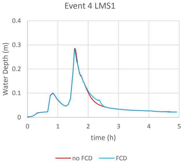
Figure 42 Event 4 water depth simulation with and without FCD at the LMS1
