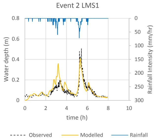
Figure 8 Comparison of water depth observed in LMS1 and modelled
