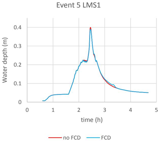
Figure 47 Event 5 water depth simulation with and without FCD at the LMS1
