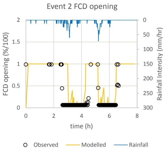
Figure 9 Comparison of modelled and observed FCD operation
