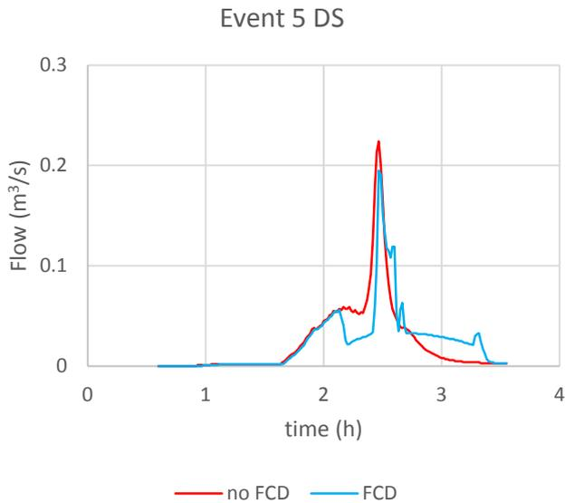
Figure 48 Event 5 flow simulation with and without FCD at the first manhole downstream the FCD
