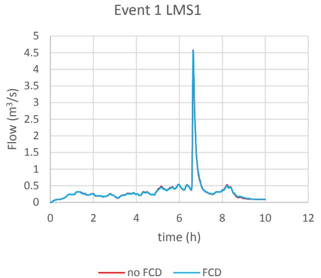
Figure 28 Event 1 flow simulation with and without FCD at the first manhole downstream the FCD
