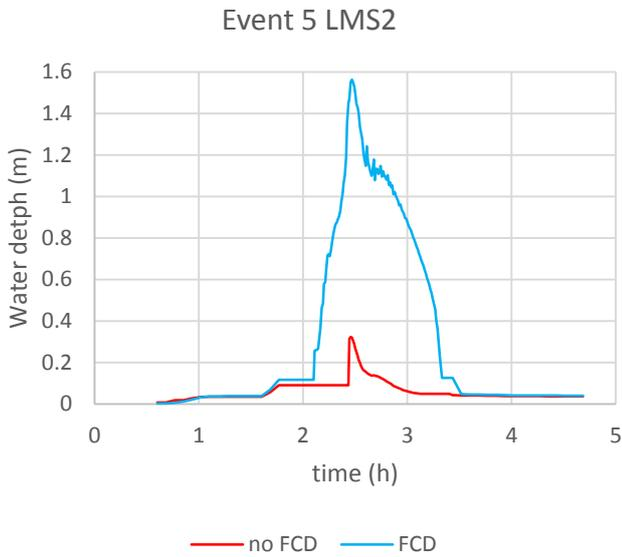
Figure 45 Event 5 water depth simulation with and without FCD at LMS2
