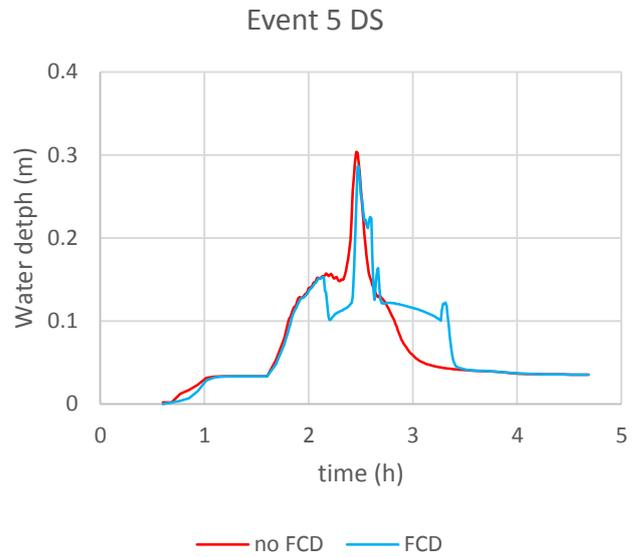
Figure 46 Event 5 water depth simulation with and without FCD at the first manhole downstream the FCD
