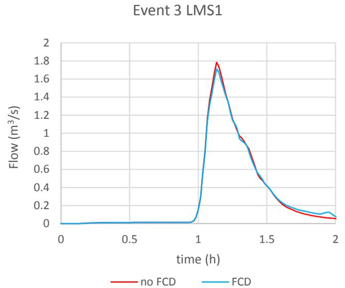
Figure 39 Event 3 flow simulation with and without FCD at the LMS1
