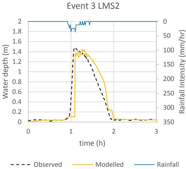
Figure 10 Comparison of water depth observed in LMS2 and modelled
