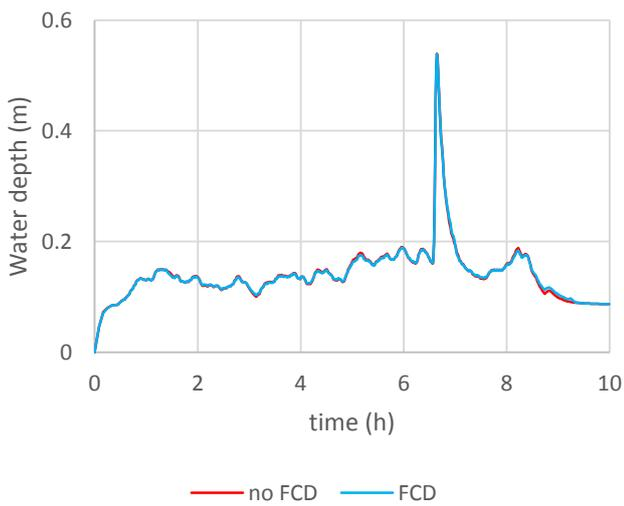
Figure 27 Event 1 water depth simulation with and without FCD at the LMS1
