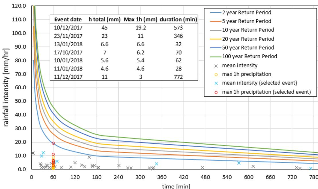
Figure 2 Intensity-Duration Curves and Data from 41 rainfall events that activated the FCD during the period of tests. Selected events, which were chosen to cover a range of rainfall depths and durations, are highlighted.
