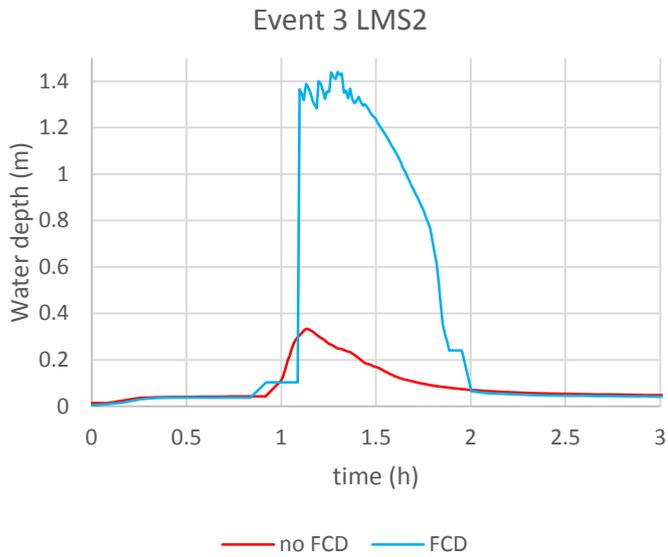
Figure 35 Event 3 water depth simulation with and without FCD at the LMS2
