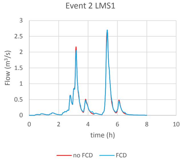
Figure 33 Event 2 flow simulation with and without FCD at the first manhole downstream the FCD
