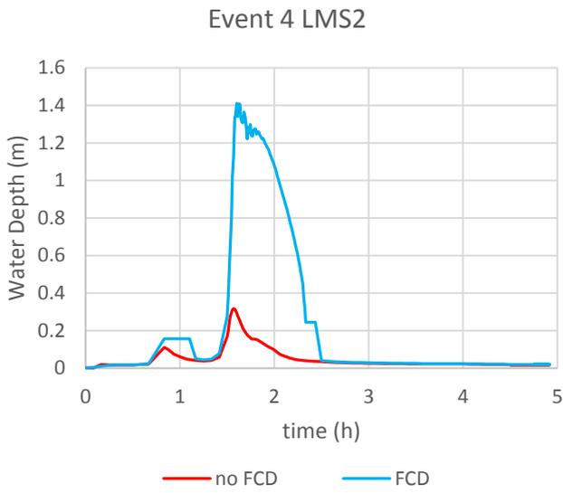
Figure 40 Event 4 water depth simulation with and without FCD at the LMS2
