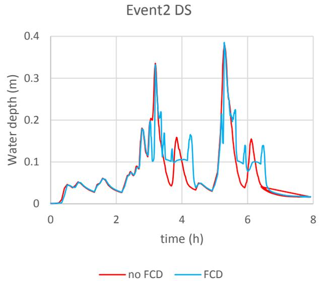
Figure 31 Event 2 water depth simulation with and without FCD at the first manhole downstream the FCD
