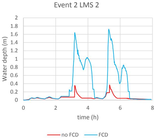
Figure 30 Event 2 water depth simulation with and without FCD at the LMS2
