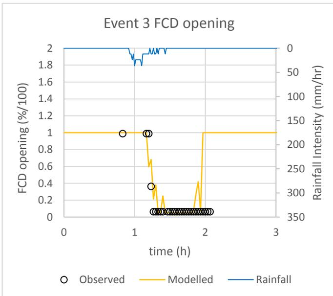
Figure 12 Comparison of modelled and observed gate operation
