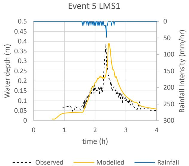
Figure 17 Comparison of water depth observed in LMS1 and modelled
