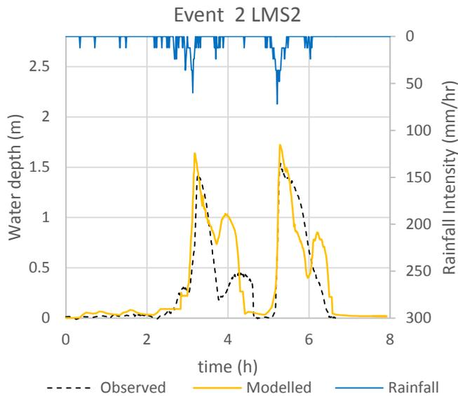
Figure 7 Comparison of water depth observed in LMS2 and modelled
