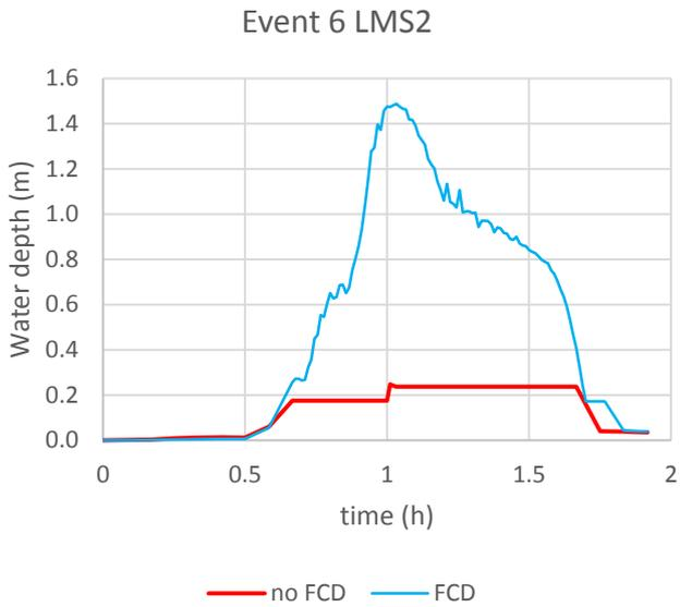
Figure 50 Event 6 water depth simulation with and without FCD at the LMS2
