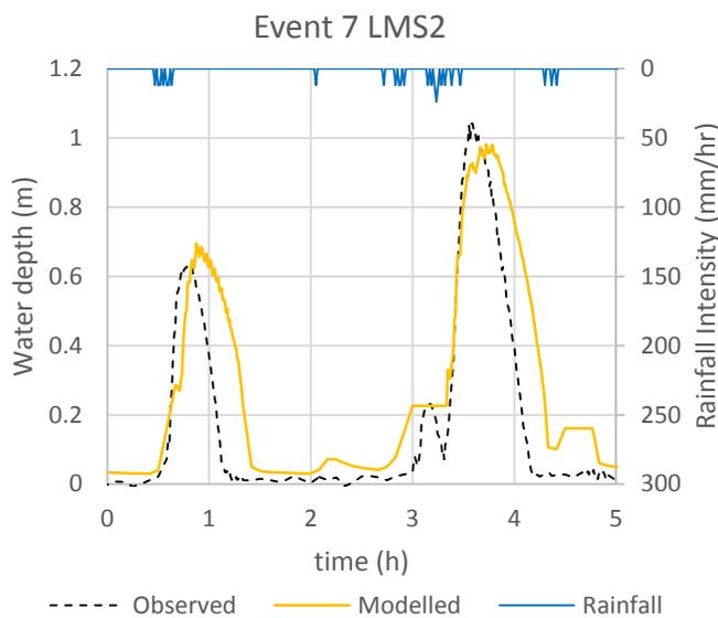
Figure 22 Comparison of water depth observed in LMS2 and modelled
