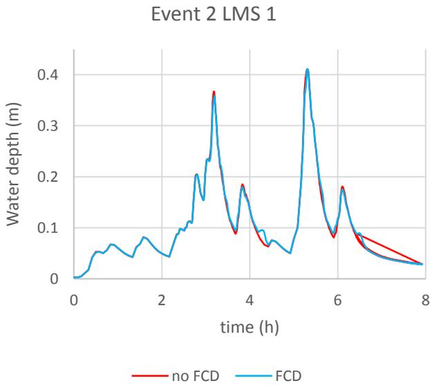
Figure 32 Event 2 water depth simulation with and without FCD at the LMS1
