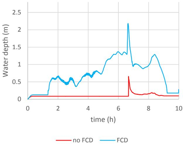
Figure 25 Event 1 water depth simulation with and without FCD at the LMS2
