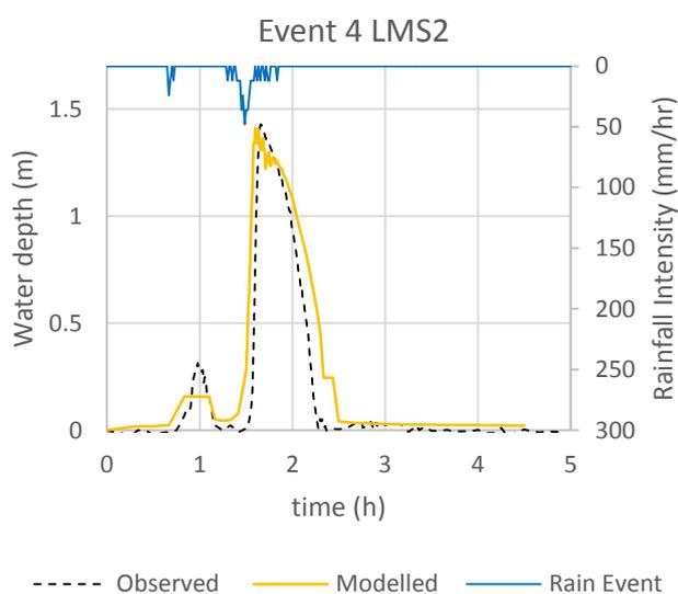
Figure 13 Comparison of water depth observed in LMS2 and modelled
