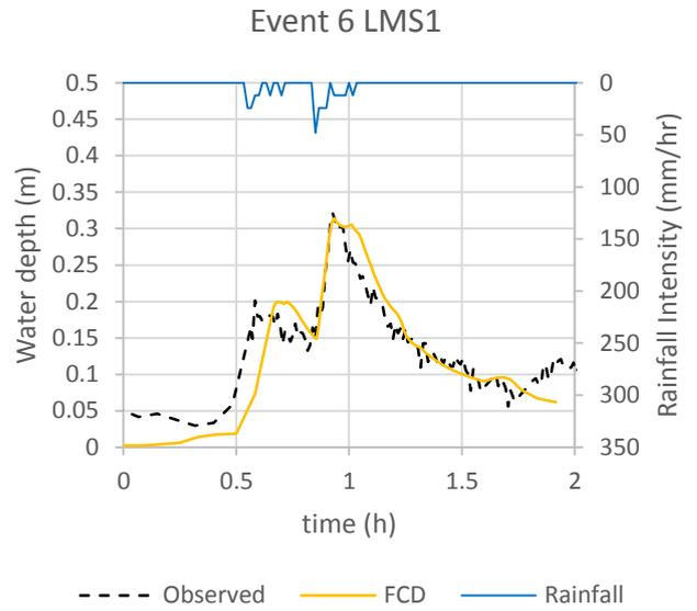
Figure 20 Comparison of water depth observed in LMS1 and modelled
