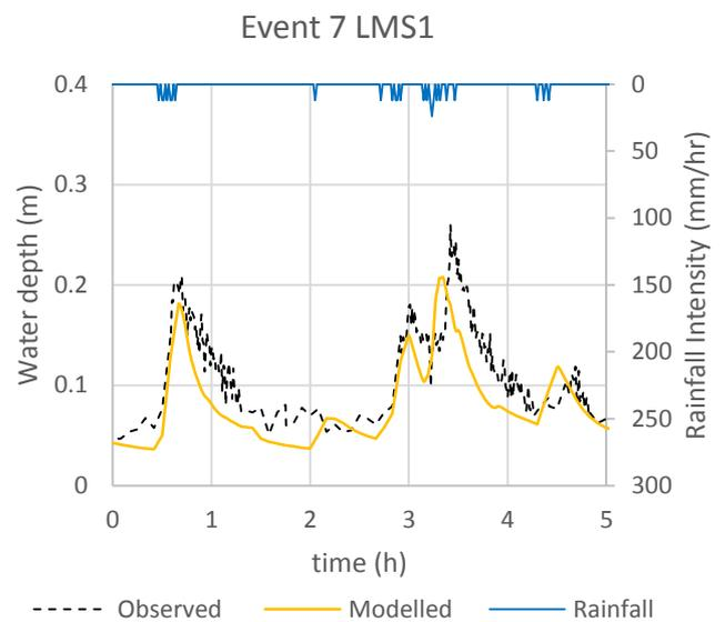
Figure 23 Comparison of water depth observed in LMS1 and modelled
