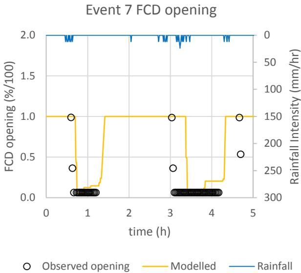
Figure 24 Comparison of modelled and observed FCD operation
