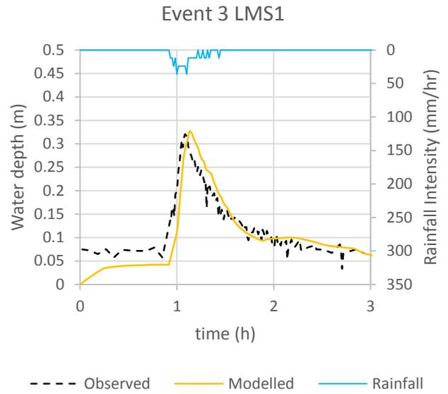
Figure 11 Comparison of water depth observed in LMS1 and modelled
