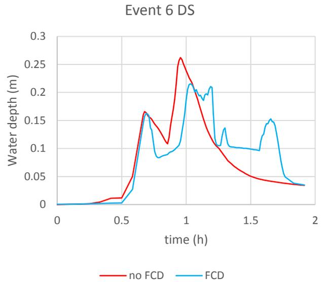
Figure 51 Event 6 water depth simulation with and without FCD at the first manhole downstream the FCD
