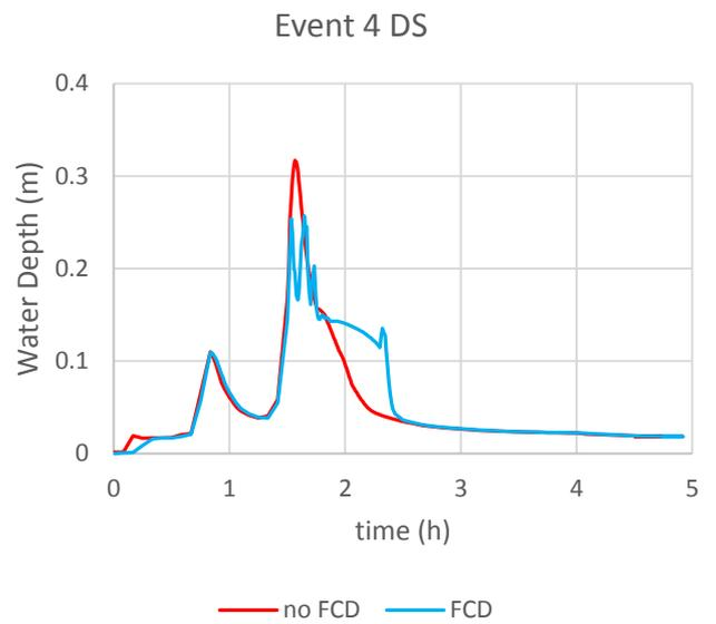
Figure 41 Event 4 water depth simulation with and without FCD at the first manhole downstream the FCD
