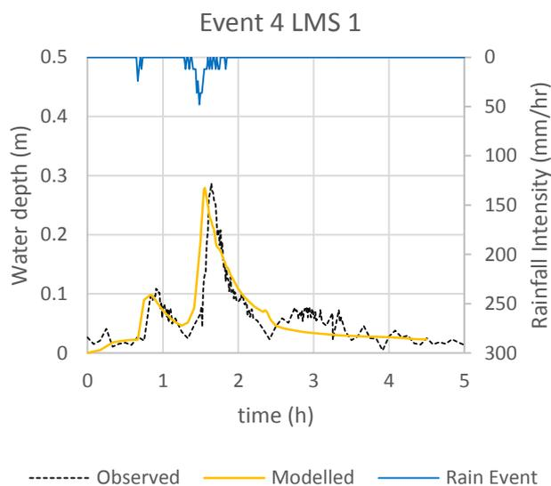
Figure 14 Comparison of water depth observed in LMS1 and modelled
