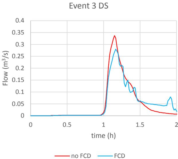
Figure 38 Event 3 flow simulation with and without FCD at the first manhole downstream the FCD
