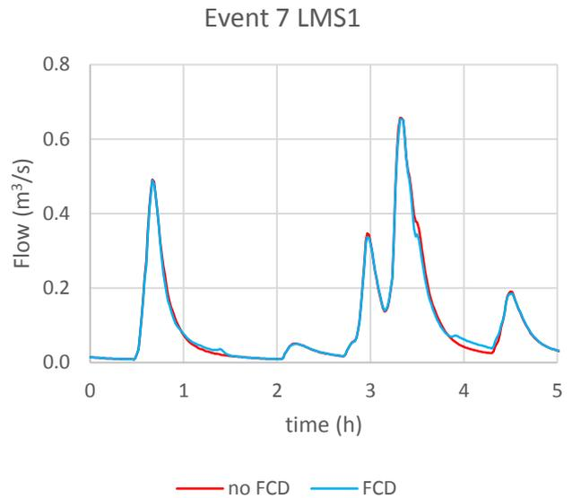
Figure 58 Event 7 flow simulation with and without FCD at the first manhole downstream the FCD
