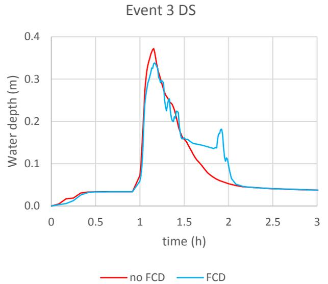
Figure 36 Event 3 water depth simulation with and without FCD at the first manhole downstream the FCD
