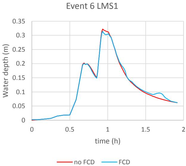
Figure 52 Event 6 water depth simulation with and without FCD at the LMS1
