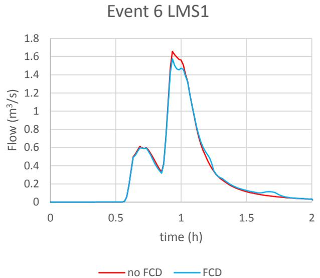
Figure 53 Event 6 flow simulation with and without FCD at the first manhole downstream the FCD
