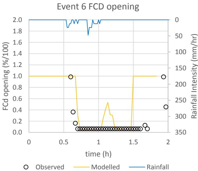
Figure 21 Comparison of modelled and observed gate operation
