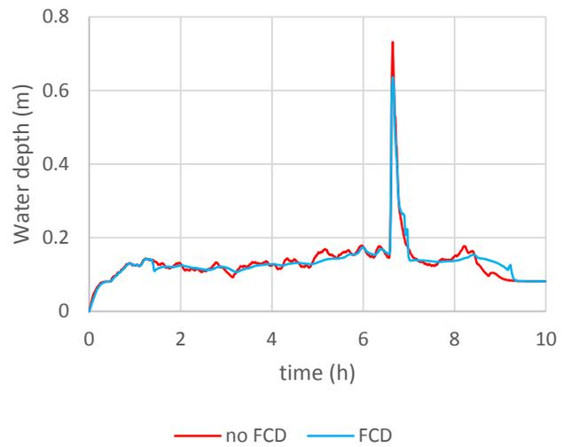
Figure 26 Event 1 water depth simulation with and without FCD at the first manhole downstream the FCD
