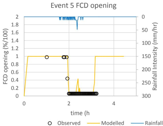
Figure 18 Comparison of modelled and observed FCD operation
