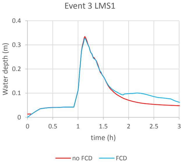
Figure 37 Event 3 water depth simulation with and without FCD at the LMS1
