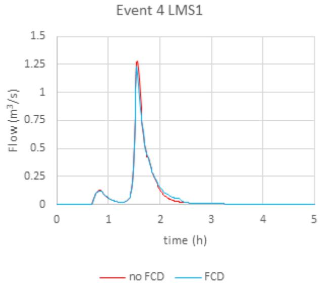
Figure 43 Event 4 flow simulation with and without FCD at the first manhole downstream the FCD
