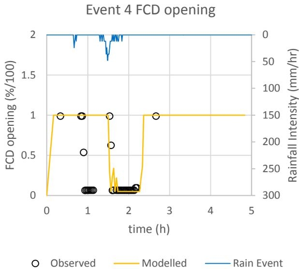
Figure 15 Comparison of modelled and observed FCD operation
