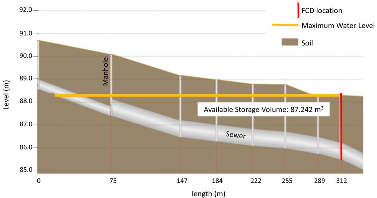
Figure 2 Longitudinal profile perspective showing the pipes available for storage (maximum water level is just below the ground surface)
