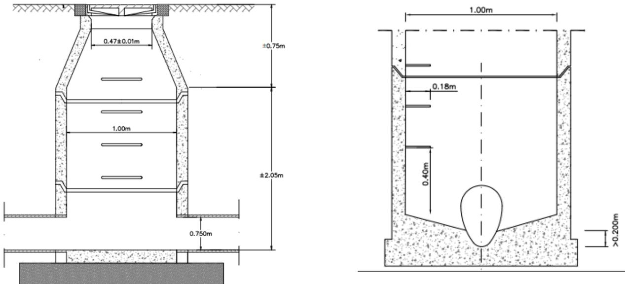
Figure 1: Geometry of selected manhole for installation of the FCD
