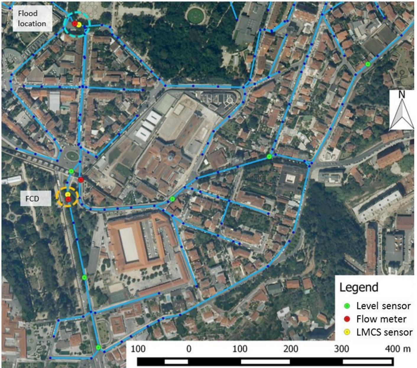
Figure 9 Location of: Monitoring sensors for testing, CENTAUR FCD, Flood Location.
