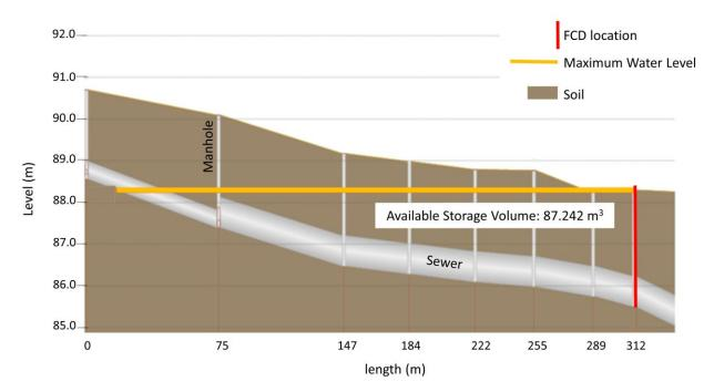
Figure 2 Longitudinal profile perspective showing the pipes available for storage (maximum water level is just below the ground surface)
