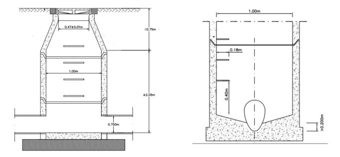
Figure 1: Geometry of selected manhole for installation of the FCD
