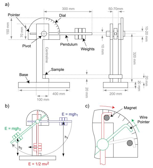
Figure 2 - a) Schematic diagram of a suitable test rig, with suggested suitable dimensions. b) A diagram of the test procedure, showing the energy present in the system at each stage. c) one suggested mechanism for recording the maximum swing in each test.
