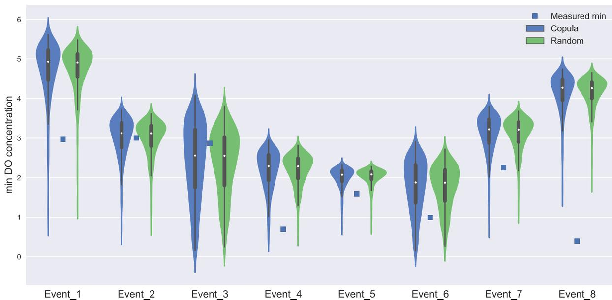
Fig 4 Minimum DO level for every event in which measurements are below 3 mg/l.
