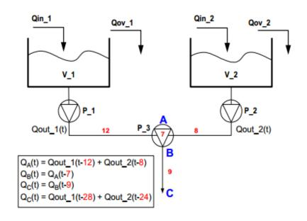
Time delay concept used in the network modelling.
