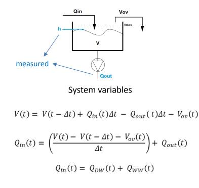
h: wastewater level in the tank (measured by sensor) Qin: inflow Vov: overflow volume V: wastewater volume in the tank Qout: outflow (measured and subject to control) C: concentration of the pollutant load in the tank
