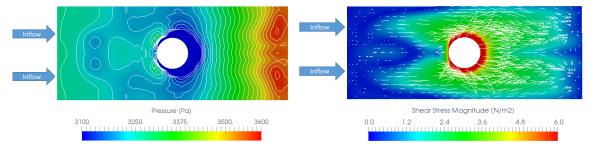
Figure 6: Pressure variation (left panel) and wall shear stress (right panel) at the bottom of the gully
