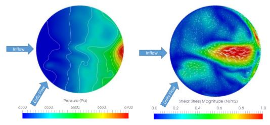
Figure 7: Pressure variation (left panel) and wall shear stress (right panel) at the bottom of the manhole
