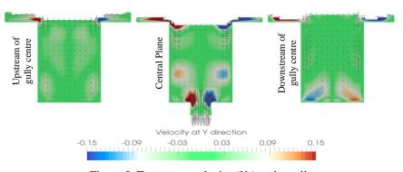
Figure 5: Transverse velocity (Vy) at the gully
