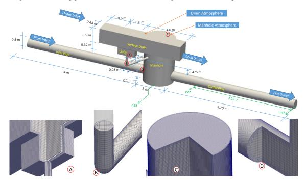
Figure 1: Upper Panel: Experimental setup; Lower panel: Computational mesh of different parts of the domain A: Gully with outlet pipe, B: Outlet Pipe, C: Manhole and D: Pipe connected with Manhole
