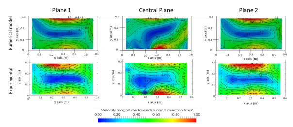
Figure 3: Comparison of velocity between numerical (upper panel) and experimental (bottom panel) study at three longitudinal planes of the gully
