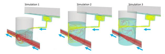
Figure 8: Flow path line / streamline inside the manhole and gully
