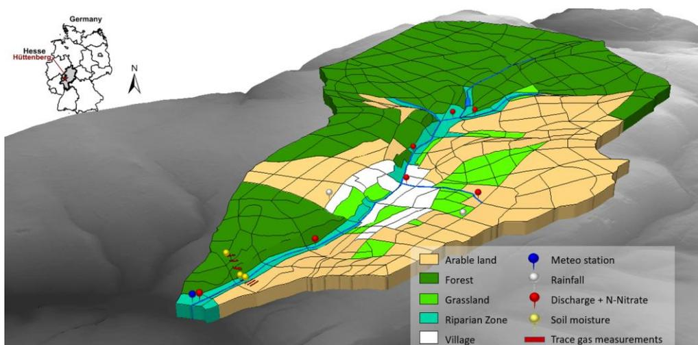
Figure 1: Digital elevation model and land use of the Vollnkirchener Bach catchment. The map shows available sampling sites and types of measurement data. Continuous high-resolution data measurements for discharge and nitrate instream are available at the catchment outlet and are used as validation data in this study.
