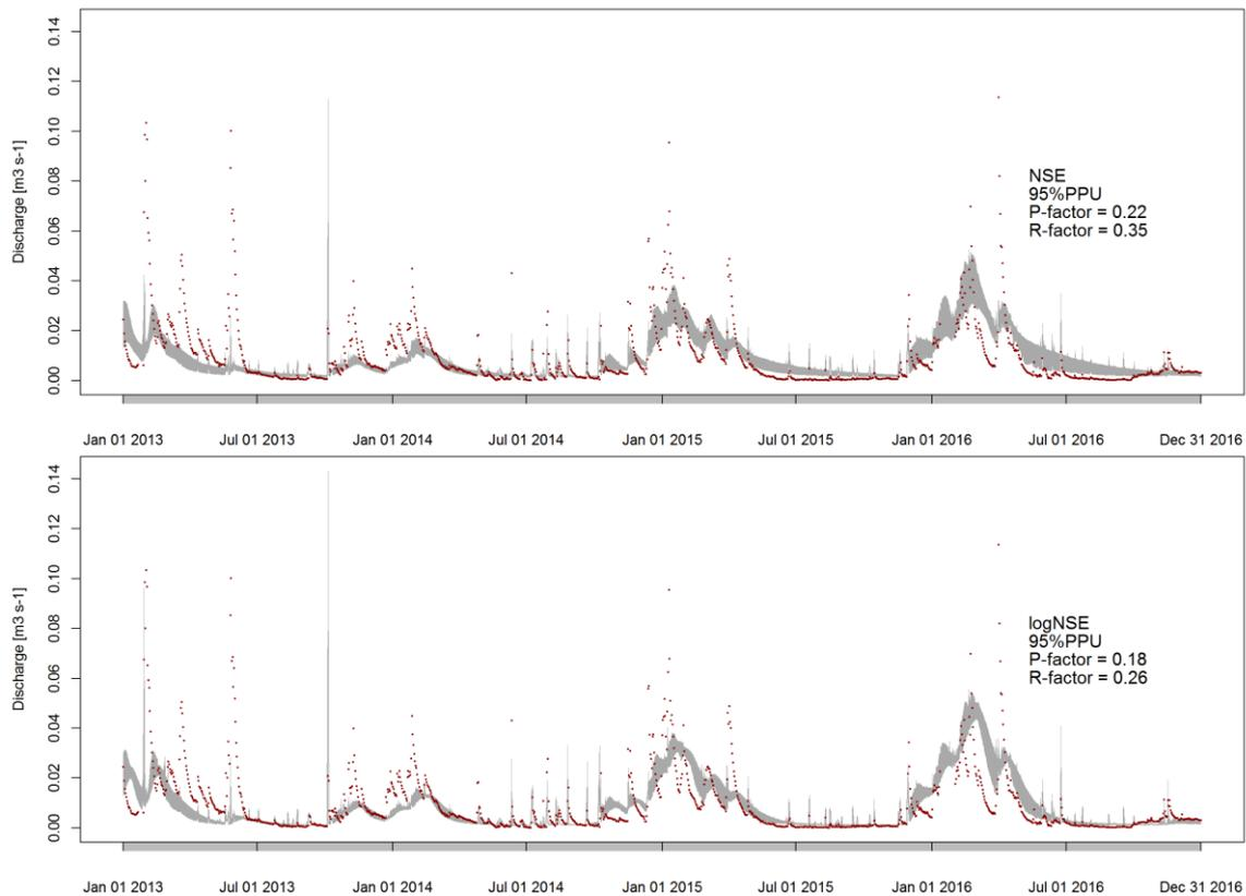
Figure 4: Hydrographs comparing the posterior model results for different goodness-of-fit criteria. The plots include the 95% prediction uncertainty, and the P- and R- factors.
