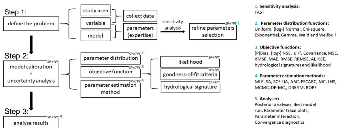
Figure 2: Calibration and uncertainty analysis three-step process. The superscripted numbers indicate the technical methods applied with the SPOTPY package (Houska et al. 2015).
