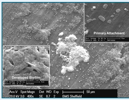
Mixed microbial species biofilms form upon the walls (Fig. 1) of drinking water distribution system (DWDS) pipelines. Biofilms adhere via extracellular polymeric substances (EPS), primarily carbohydrates and proteins, produced by microorganisms. The EPS provides physical stability to the biofilm. If the adhesive forces are overcome by shear stresses at the pipe wall, biofilm becomes mobilised into the bulk water, degrading water quality.
