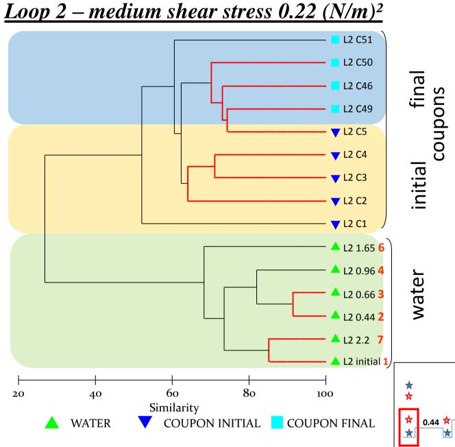
► Bray-Curtis similarity analysis (Fig. 6), clearly separated the coupon samples before flushing, from those after flushing and from bulk water samples obtained at different shear stress's during the discolouration event.
