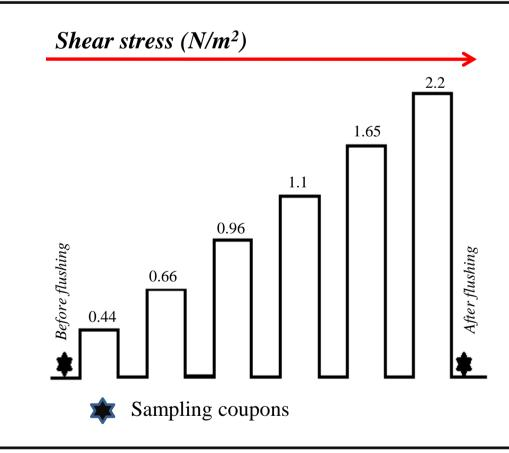
Fig. 3: Incremental shear stress applied to each loop after 28 days biofilm development.
