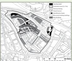
A flood channel bisecting the site provides flood protection up to the 1 in 100 year flood event and additional greenspace.
