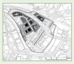
New buildings are kept within existing grid structure and are stepped in height; from 2 storeys, close to the river, to 5 storeys.
