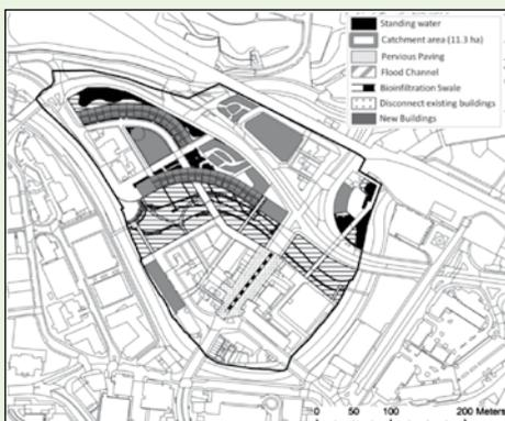
A flood channel bisecting the site provides flood protection up to the 1 in 100 year flood event and additional greenspace.
