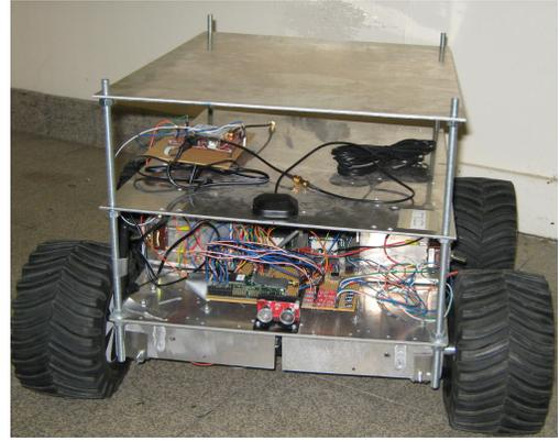
Figure 2. Autonomous Ground Vehicle (AGV)
