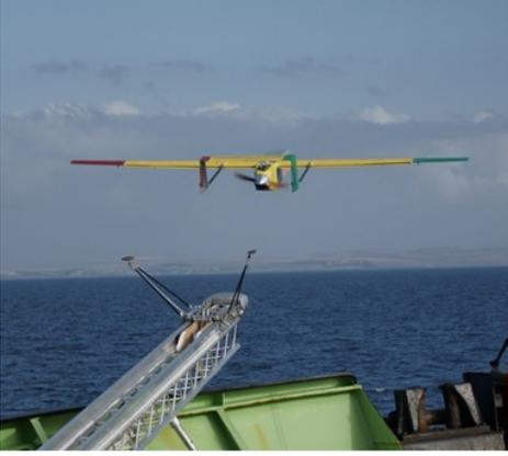
Figure 1. NOC UAV launched from research ship
