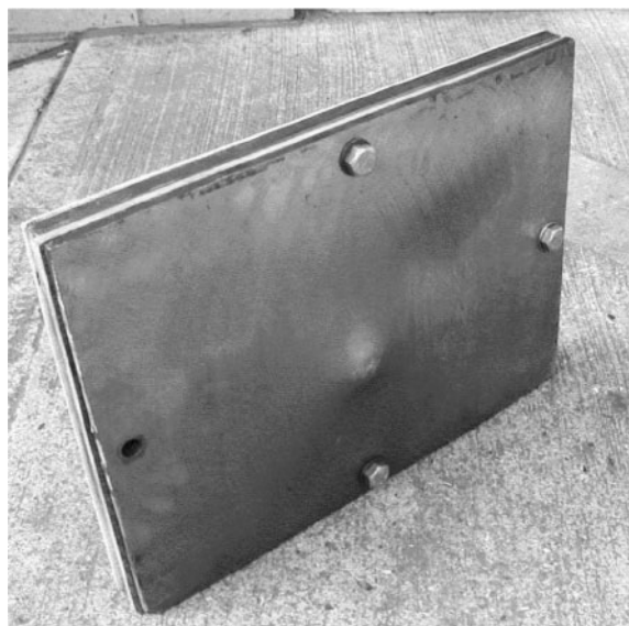
9 Result of ballistic test on Fe-0.98C-1.46Si-1.89Mn-0.26Mo-1.26Cr-0.09V, transformed at 200°C for 5 days: rear view, showing lack of penetration (courtesy D. Crowther and P. Brown)
