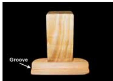
Underside of the sliding block, showing position of edge piece with groove forming a projecting 'lip'.
