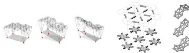
Figure 4. Testing the adaptability of the pavilion on different water level and structure behaviour of the super-structure layer.
