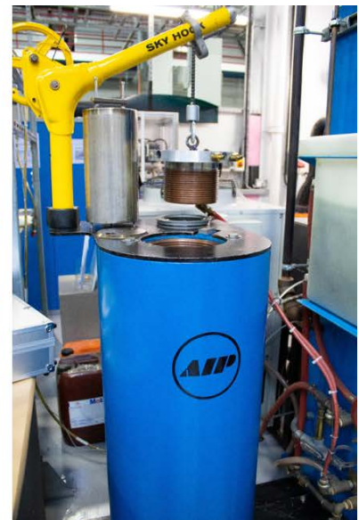
Photographs of the active furnace isolation chamber, locking station and transport case (left) and the nuclear research hot isostatic press (right)
